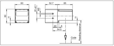
Figure 3.4: Dimensions of the angle housing
