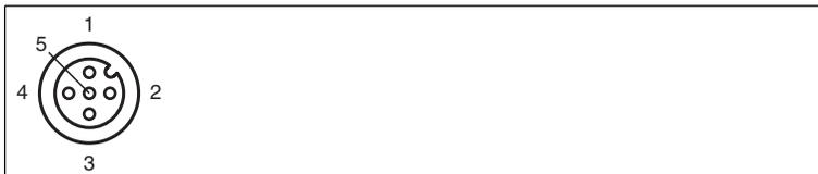
Figure 4.7 RS 232 connection layout
