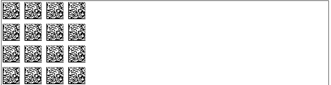
Figure 8.14 The code card automatically assigns the orientation 0°, 90°, 180°, or 270° to the read head.
