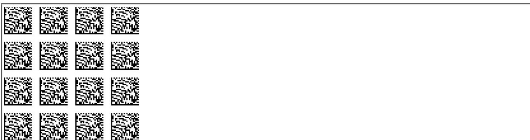
Figure 8.10 The code card assigns a position data resolution of 0.1 mm / 1 mm / 10 mm to the reading head.
