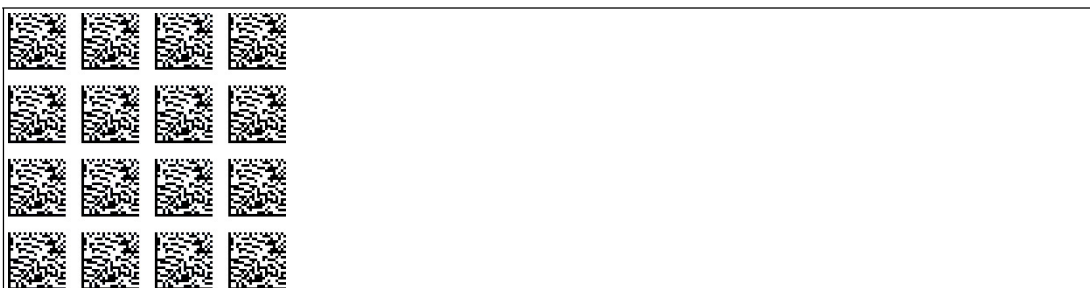
Figure 8.11 The code card assigns the orientation 0° to the read head.
