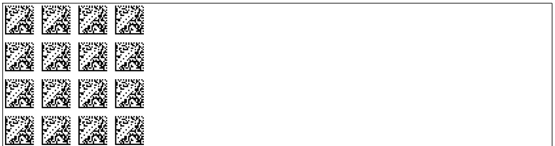
Figure 8.1 The code card "ENABLE" is used to activate external parameterization operating mode.
