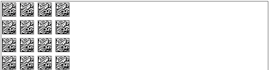
Figure 8.8 The code card assigns a position data resolution of 0.1 mm / 1 mm / 10 mm to the reading head.
