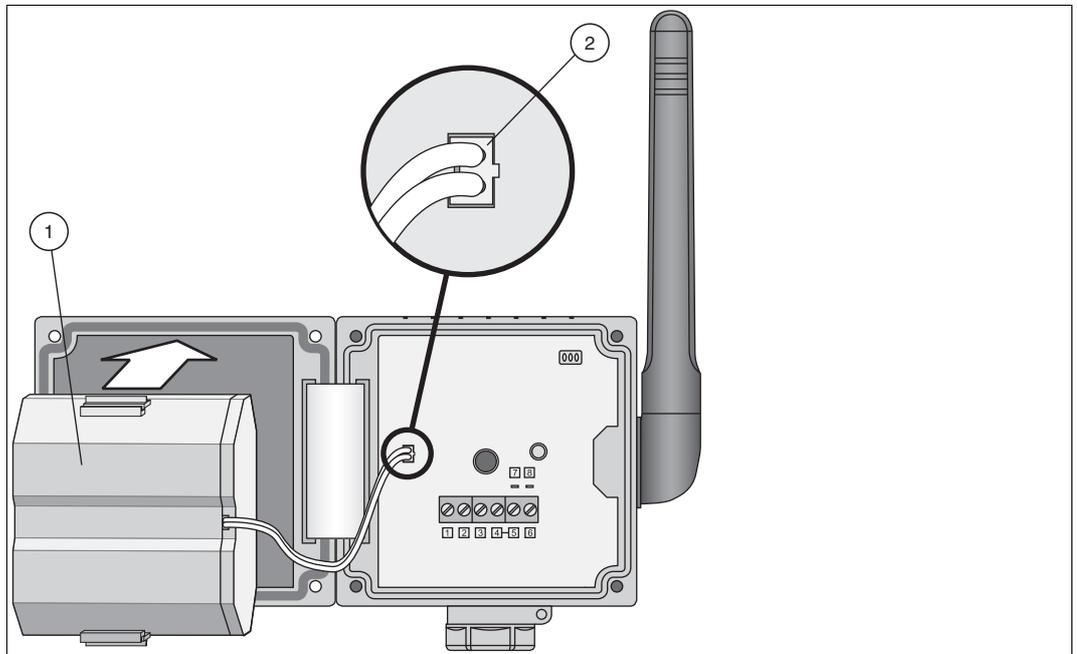
Figure 2.2 Inserting and connecting the battery
