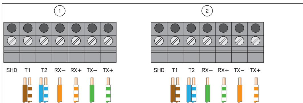
Figure 1.3 Connecting an Ethernet cable to the Ethernet terminal block
