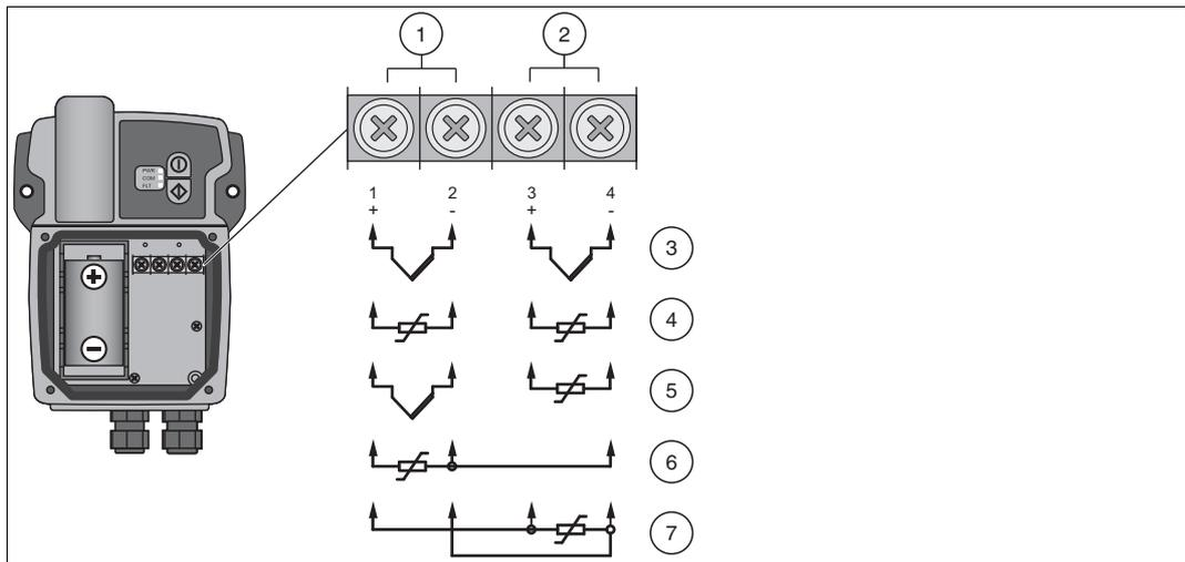
Figure 3.1 Connecting RTDs and/or TCs to the sensor interface
