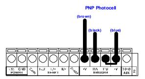
Figure 115 - External Trigger Using CBX800 Power
