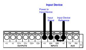
Figure 29 - PNP Input 2 Using CBX800 Power
