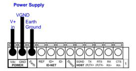
Figure 22 - Power Supply Connections
