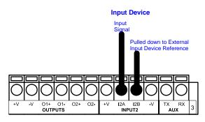
Figure 13 - PNP Input 2 Using External Power
