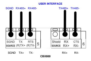
Figure 21 - RS485 Full-duplex Connections
