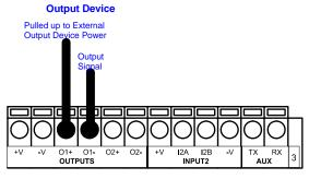
Figure 17 - Output Open Emitter Using External Power
