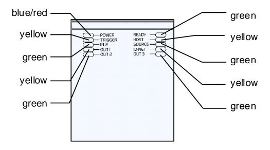
Figure 19 - Indicator LEDs
