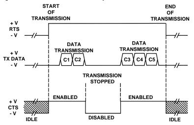
Figure 55 - RS232 Control Signals
