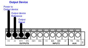
Figure 16 - Open Collector Output Using CBX800 Power
