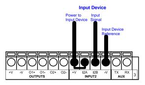
Figure 30 - NPN Input 2 Using CBX800 Power
