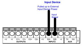
Figure 14 - NPN Input 2 Using External Power
