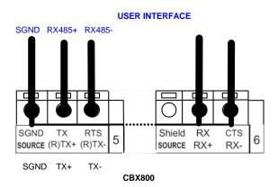
Figure 82 - RS485 Full-duplex Connections using Only TX Signals
