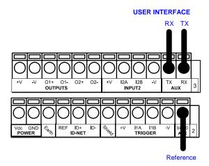
Figure 19 - RS232 Auxiliary Interface Connections
