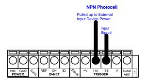
Figure 28 - NPN External Trigger Using External Power
