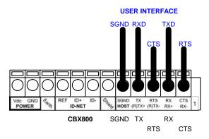
Figure 44 - RS232 Host Interface Connections Using Hardware Handshaking
