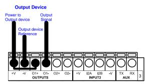
Figure 15 - Open Emitter Output Using CBX800 Power
