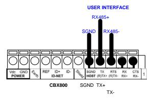
Figure 77 - RS485 Full-duplex Connections using Only TX Signals
