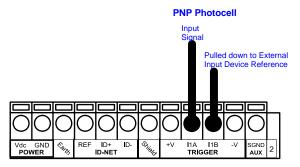
Figure 27 - PNP External Trigger Using External Power
