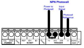
Figure 126 - NPN External Trigger Using CBX800 Power
