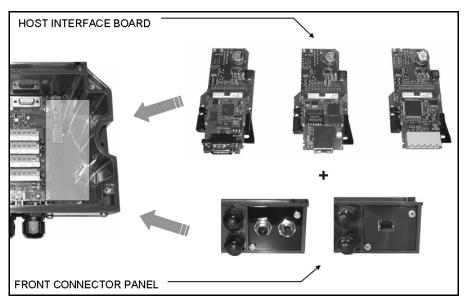
Figure 1 - CBX800 Front Connector Panel
