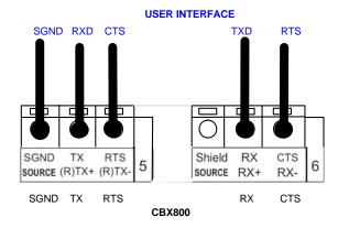
Figure 20 – RS232 Data Source Interface Connections
