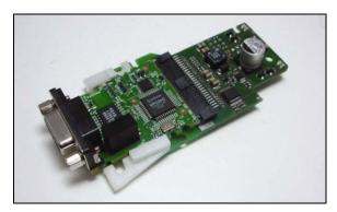
Figure 34 - Host Interface Module
