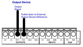
Figure 18 - Output Open Collector Using External Power
