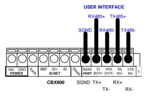
Figure 66 - RS485 Full-duplex Connections
