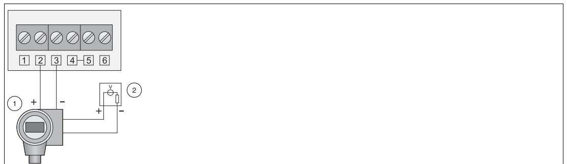
Figure 3.15 Connection of active four-wire device to passive adapter
