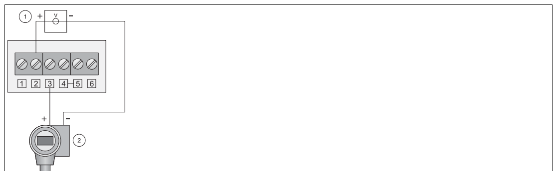
Figure 3.11 Alternative method of connection of adapter to a control loop without communication resistor
