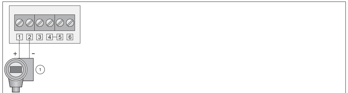
Figure 3.14 Connection of loop-powered device to active adapter
