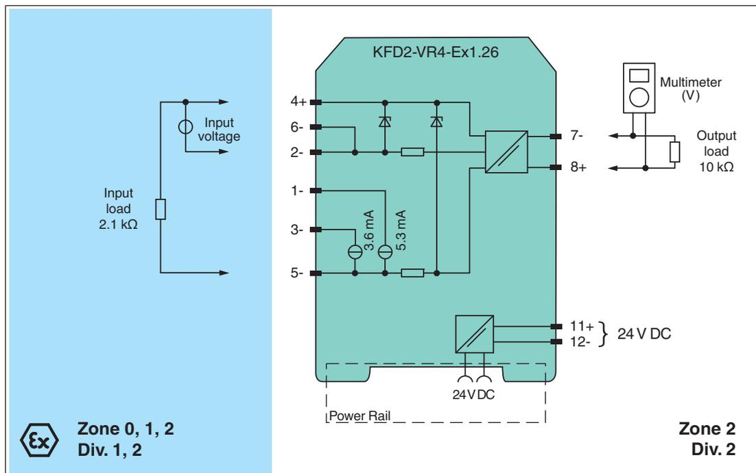
Figure 5.1 Set-up for proof tests A and B
