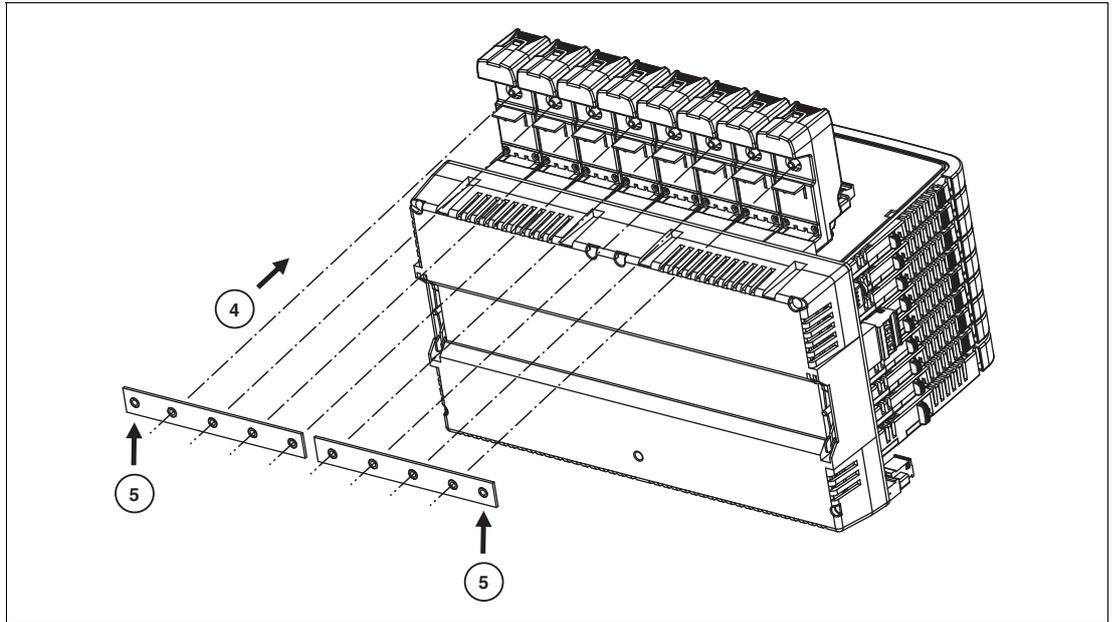
Figure 3.3 Mounting on rotated 8-channel motherboards (\*-8R.R)
