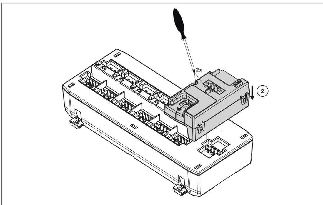
3. Plug the T-connector in the trunk connection of the Surge Protector and fix the T-connector with the 2 screws (3).
