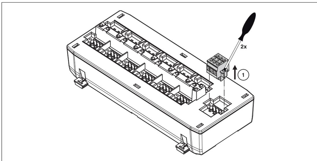
2. Plug the Surge Protector in the trunk connection and fix the Surge Protector with the 2 screws on the Segment Protector (2).
