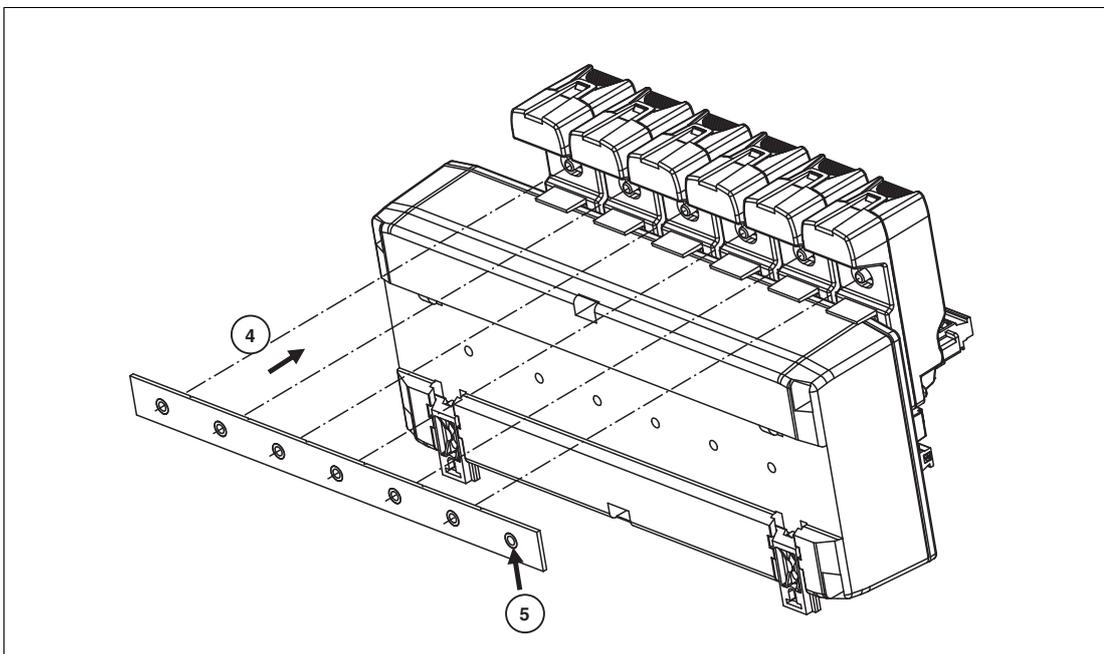
5. Connect the grounding rail to the grounding terminal of the housing (5).
