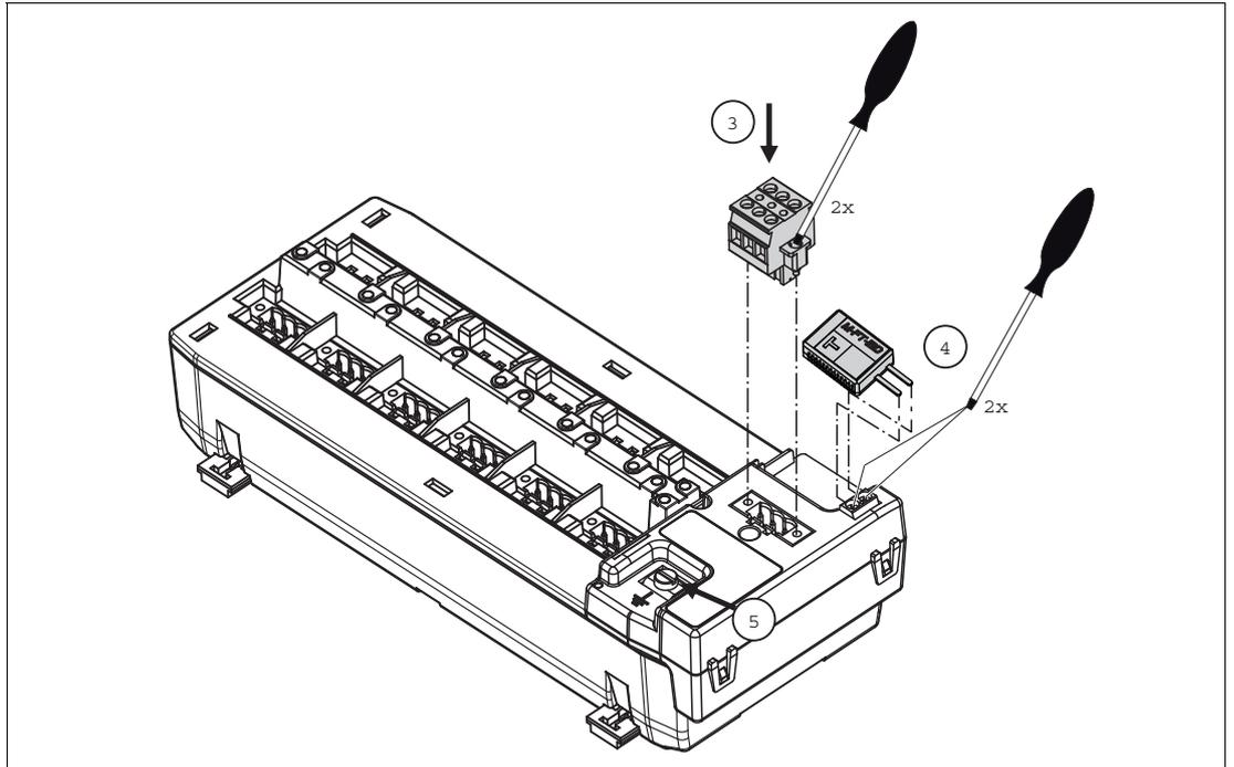
The grounding terminal should be connected to an equal potential bonding system using a minimum cross core section of 4 mm<sup>2</sup>.
