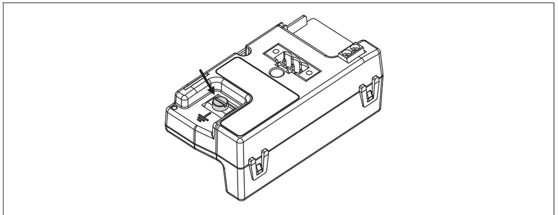
The shield connection of the trunk is internally indirectly connected to the grounding terminal through a gas discharge tube.
