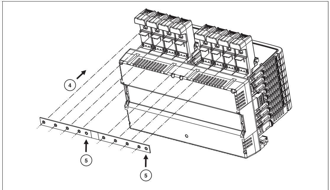
Figure 3.1 Mounting on 8-channel motherboards (\*-8R)
