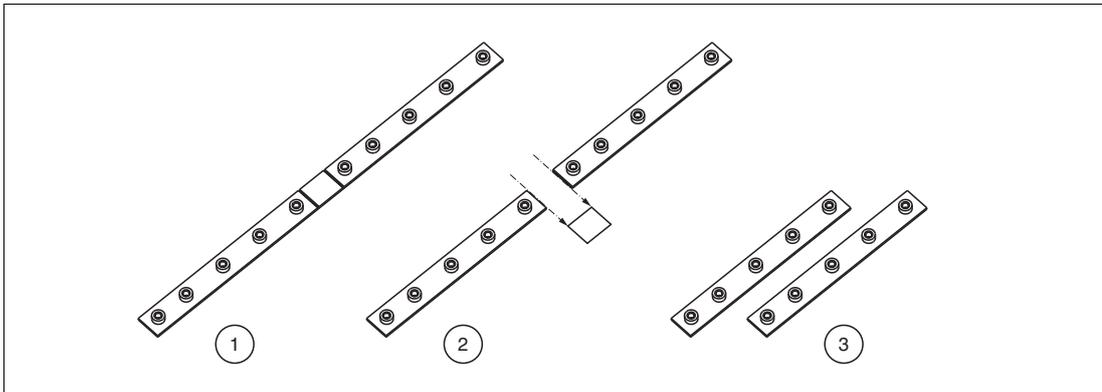
Figure 3.2 Preparation of the grounding rail mounting
