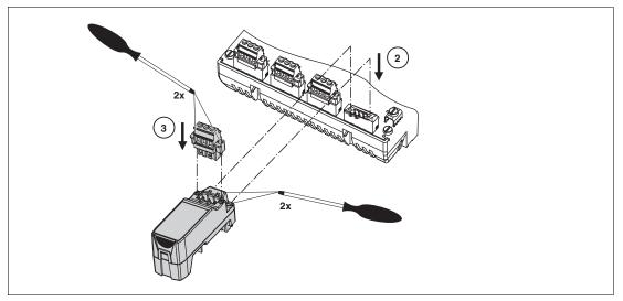
**4.** Mount the grounding rail in 2 parts on the motherboard. Separate the grounding rail and rotate one of them before mounting, see figure.
