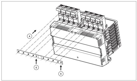
Figure 3.1 Mounting on 8-channel motherboards (\*-8R)
