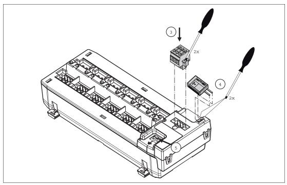
The grounding terminal should be connected to an equal potential bonding system using a minimum cross core section of  $4~\mathrm{mm}^2$ .
