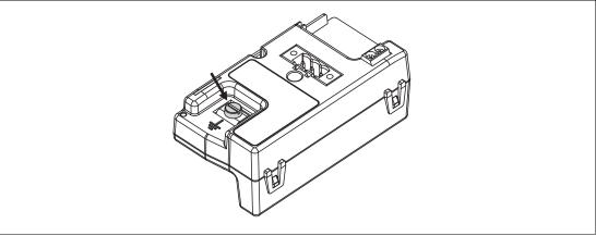
The shield connection of the trunk is internally indirectly connected to the grounding terminal through a gas discharge tube.
