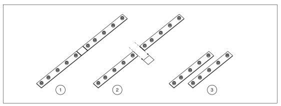
Figure 3.2 Preparation of the grounding rail mounting
