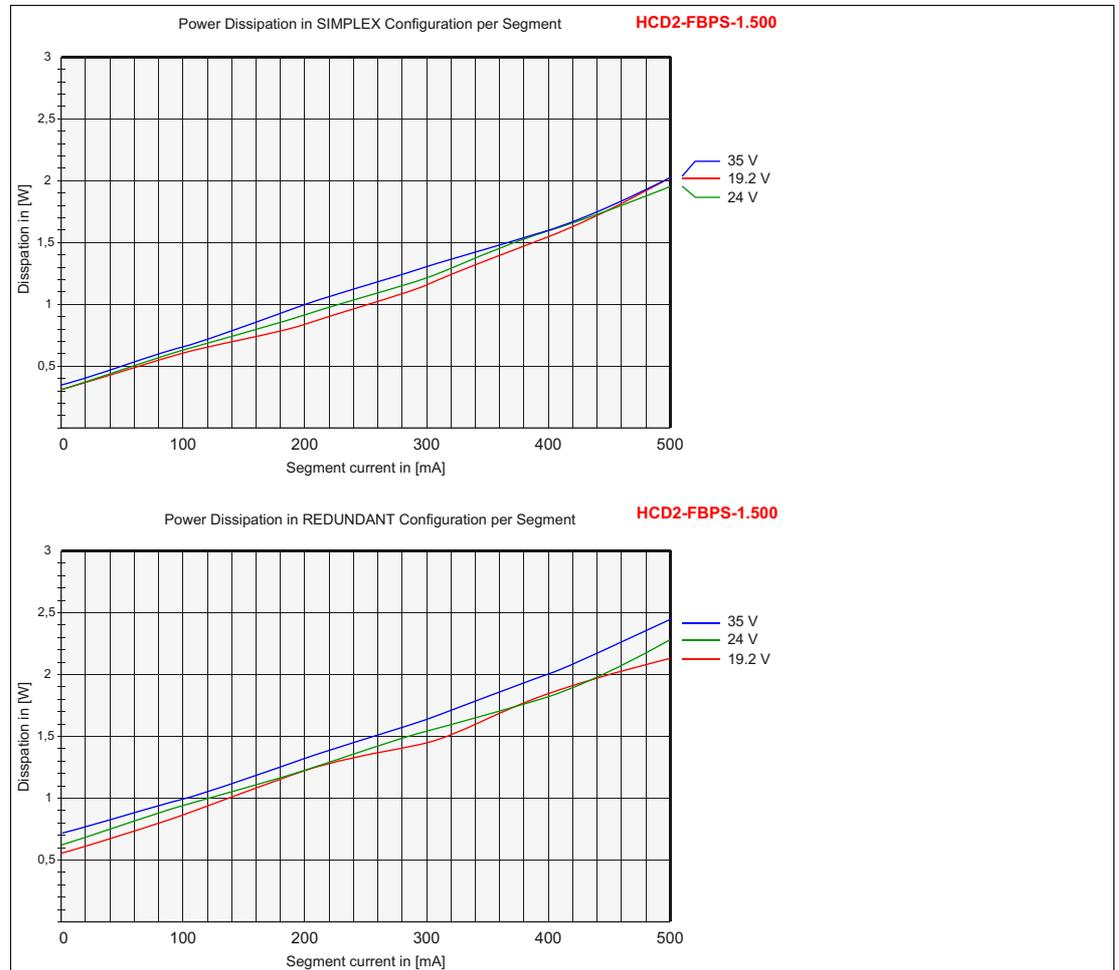
**Thermal Dissipation of HCD2-FBPS-1.23.500, Including Motherboard**
