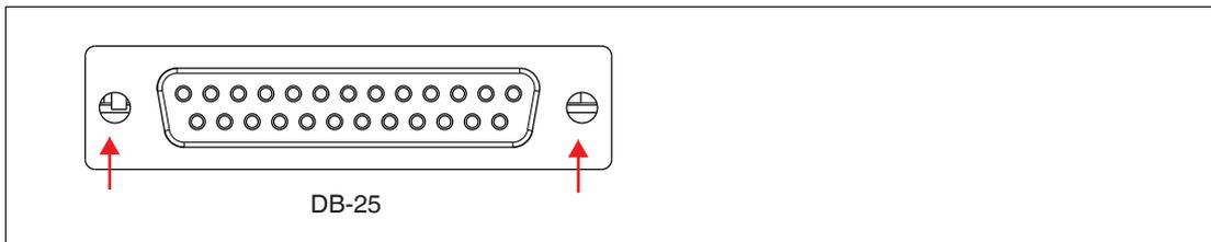
In order to fasten the male connector onto the female D-Sub 25 pin connection: Turn each of the 2 jack screws of the connector until the connector is connected tightly with the socket. In order to check that the connector is fastened properly and cannot come off: Gently pull at the connector cable. Adjust the screws if needed.
