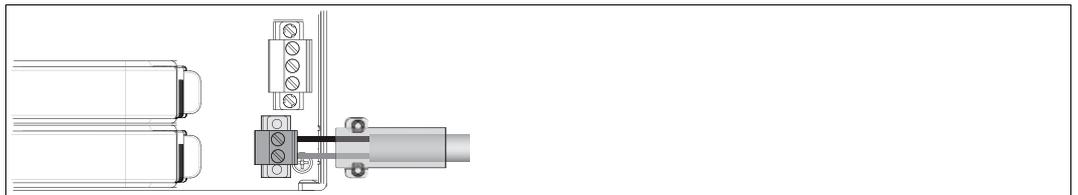
4. Put the connector cover over the power supply connector and tighten the fastening screws.
