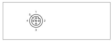
Figure 4.8 RS-232 connection layout
