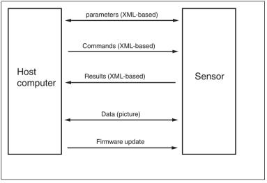
Figure 11.1 Network interface XML-Stings
