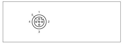
Figure 4.4 RS-232 input connection layout
