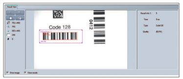
9. Enter the code to be compared under Match Code in the 1D/2D Parameter menu item of the Window 1 configuration window. You can adopt a previously read code via the Use last decode button.
