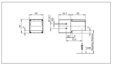
Figure 5.1 Dimensions of the **angle** housing
