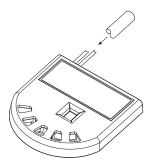
The ELS-1 comprises 2 connection lines, each 180 mm long. The sensor connection lines may be extended up to a length of 1 m. The dielectric strength of the insulation must be at least 500 V according to IEC 60079-14.
