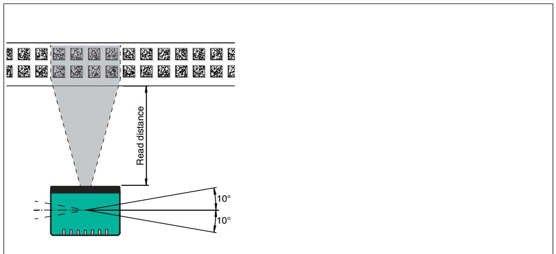
Figure 5.5 Horizontal alignment tolerance
