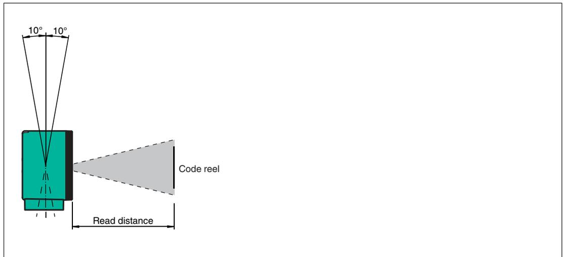
Figure 5.4 Vertical alignment tolerance
