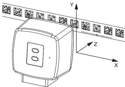
**Z coordinate:** If the distance of the camera to the code reel is too small, the yellow LED5 lights up. If the distance is too great, the yellow LED5 goes out. The yellow LED5 flashes at the same time as the green LED2 when within the target range.
