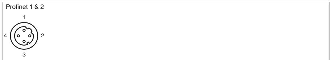
Figure 5.10 PROFINET connector assignment
