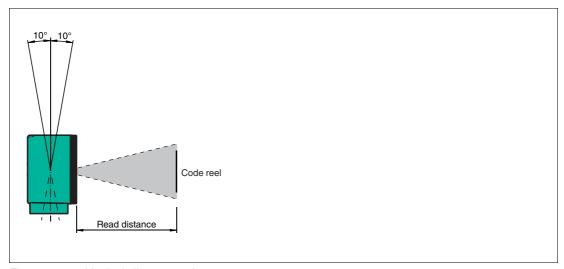
Figure 5.4 Vertical alignment tolerance
