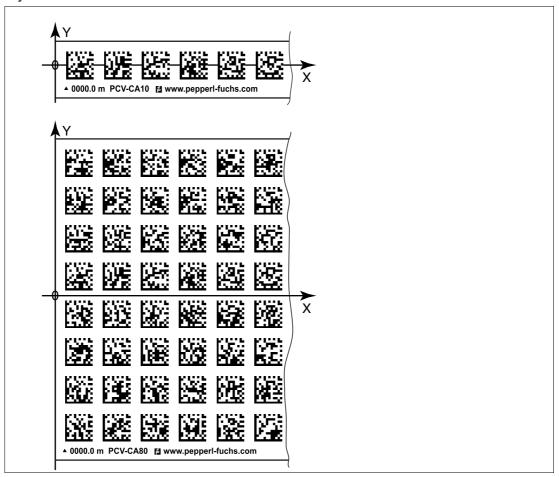
Figure 5.3 Zero line for code reels
