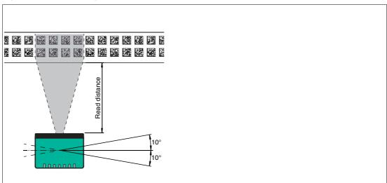
Figure 5.5 Horizontal alignment tolerance
