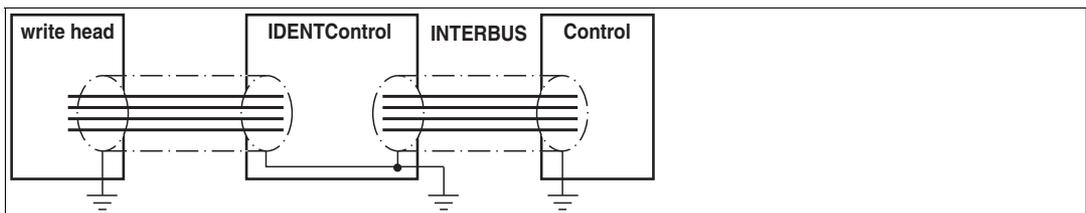
The cable shielding is used to discharge electromagnetic interference. When shielding a cable, you must connect both sides of the shield to ground with low resistance and low inductance.
