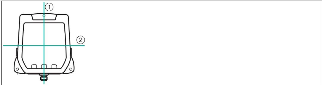
Figure 5.3      ① = Vertical polarization plane
