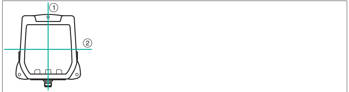
Figure 4.3 1 = Vertical polarization plane 2 = Horizontal polarization plane
