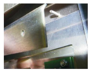
6) Before fully tightening nuts to lock bracket in place, check the front side to make sure there are no gaps, and that the keyboard is centered properly into the cut-out.
