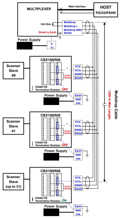
Figure 26 - VB24 Multidrop Connection to a Multiplexer
