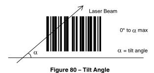
The decoder will be able to read the label with a tilt angle between  $+ \square \max and \square \max as shown in the following figure:$
