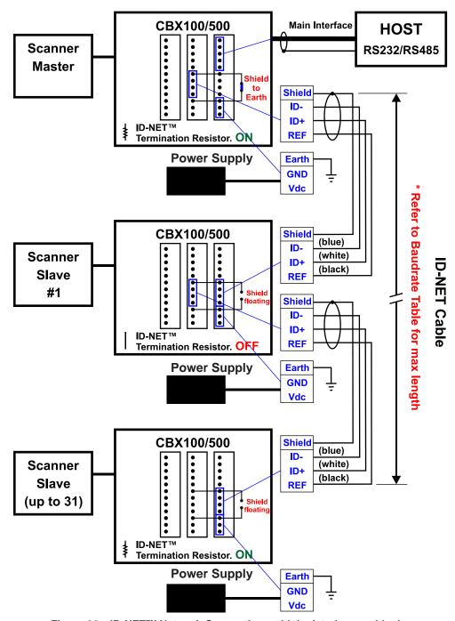
Figure 28 – ID-NET™ Network Connections with isolated power blocks
