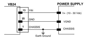
Figure 44 - Power Supply Connections
