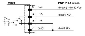
Figure 56 - PH-1 Photocell (PNP) External Trigger Using VB24 Power
