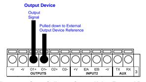
Figure 42 - Open Collector Output Using External Power
