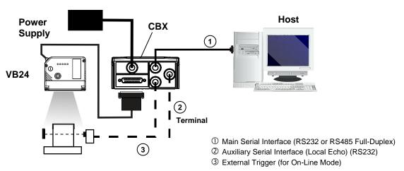
Figure 67 - Serial Interface Point-to-Point Layout
