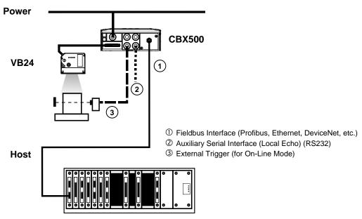
Figure 68 - Fieldbus Interface Point-to-Point Layout
