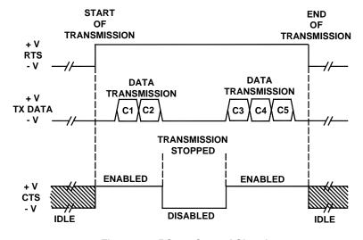
Figure 46 - RS232 Control Signals
