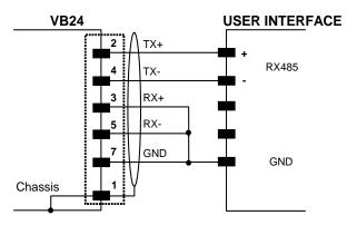
Figure 48 - RS485 Full-duplex Connections using Only TX Signals
