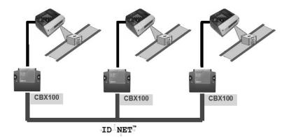
ID-NET™ interface allows connection of scanners reading objects placed on independent conveyors. All scanners are typically located far away from each other and they use a dedicated presence sensor.
