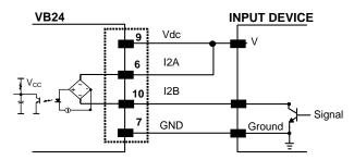
Figure 62 - NPN Input 2 Using VB24 Power
