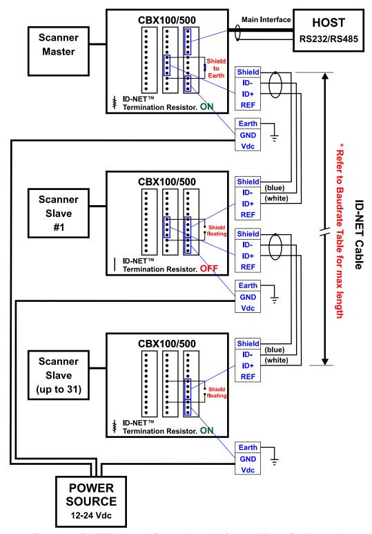
Figure 30 – ID-NET™ Network Connections with Common Power Star Network
