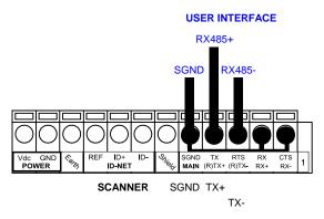
Figure 24 - RS485 Full-duplex Connections using Only TX Signals
