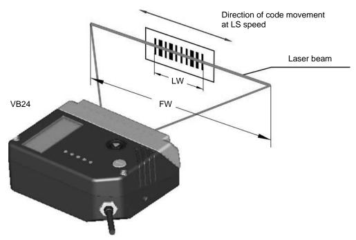
Figure 83 - "Picket-Fence" Scanning Mode
