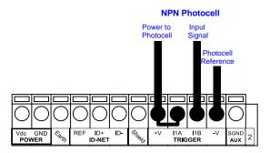
Figure 34 - NPN External Trigger Using VB24 Power
