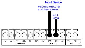
Figure 38 - NPN Input 2 Using External Power
