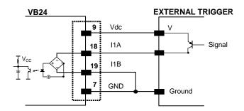
Figure 57 - PNP External Trigger Using VB24 Power
