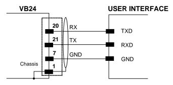
Figure 55 - RS232 Auxiliary Interface Connections
