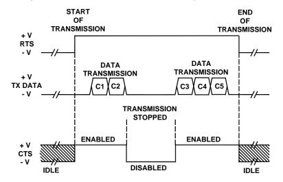
Figure 22 - RS232 Control Signals
