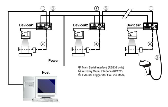
Figure 69 - Pass-Through Layout
