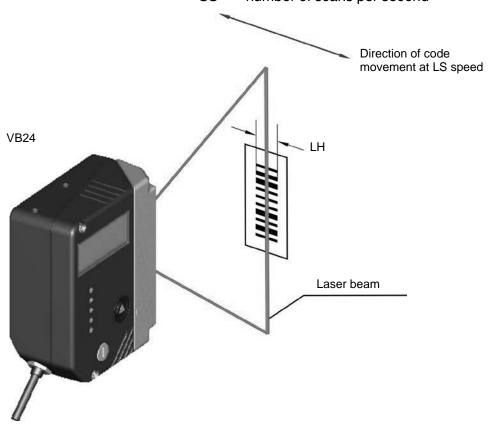
Figure 82 - "Step-Ladder" Scanning Mode
