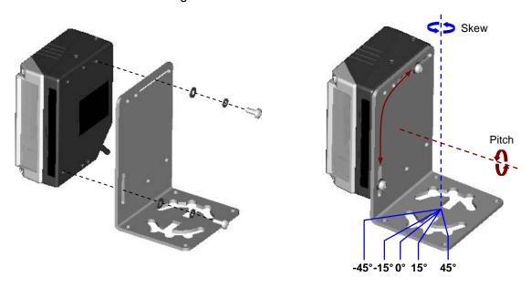
Figure 3 - Positioning with Mounting Bracket
