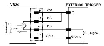
Figure 58 - NPN External Trigger using VB24 power
