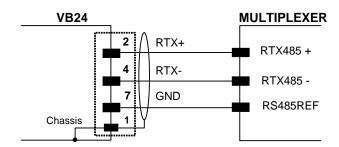
Figure 49 - RS485 Half-duplex Connections
