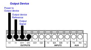
Figure 40 - Open Collector Output Using VB24 Power
