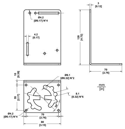
Figure 13 - L Shape Mounting Bracket Overall Dimensions
