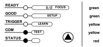
Figure 9 - Mode Interface: Test Mode Function
