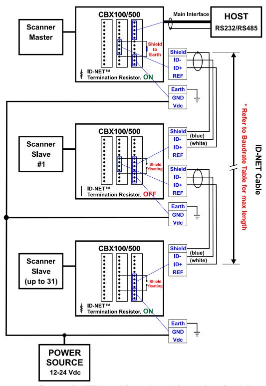
Figure 29 - ID-NET™ Network Connections with Common Power Branch Network
