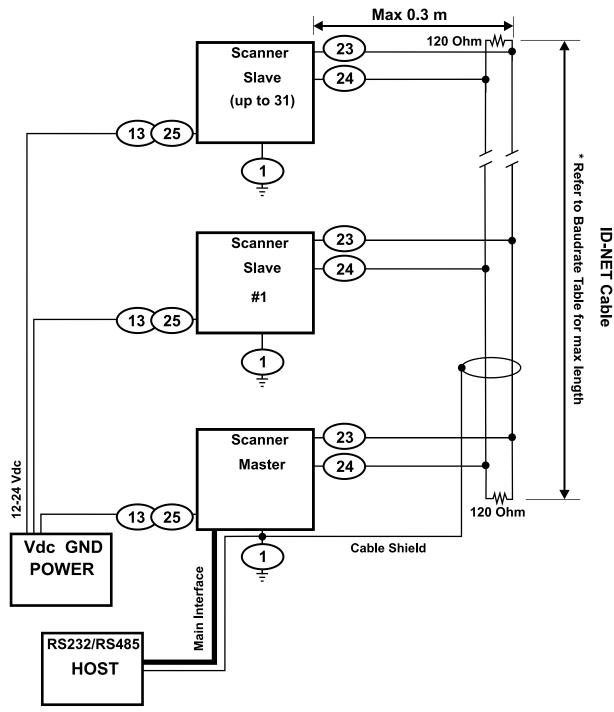
Figure 54 – ID-NET™ Network Connections with Common Power Star Network
