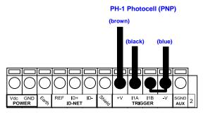
Figure 33 – PH-1 Photocell (PNP) External Trigger Using VB24 Power
