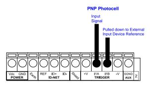
Figure 35 - PNP External Trigger Using External Power
