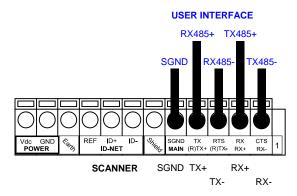
Figure 23 - RS485 Full-duplex Connections
