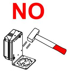
do not weld the scanner into position which can cause electrostatic, heat or output window damage.
