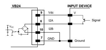
Figure 61 - PNP Input 2 Using VB24 Power
