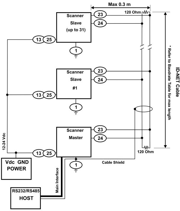
Figure 53 - ID-NET™ Network Connections with Common Power Branch Network
