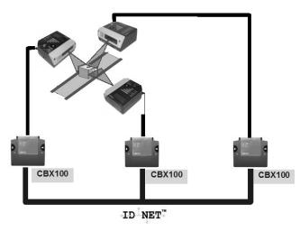
ID-NET™ interface allows local connection of multiple scanners reading different sides of the same target. All scanners share a single presence sensor and activate/deactivate simultaneously.
