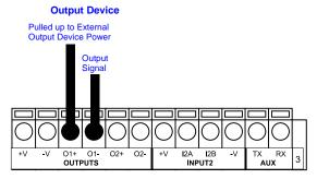
Figure 41 - Open Emitter Output Using External Power
