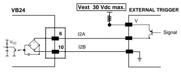
Figure 63 - PNP Input 2 Using External Power
