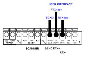
Figure 25 - RS485 Half-duplex Connections
