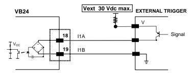
Figure 59 - PNP External Trigger Using External Power
