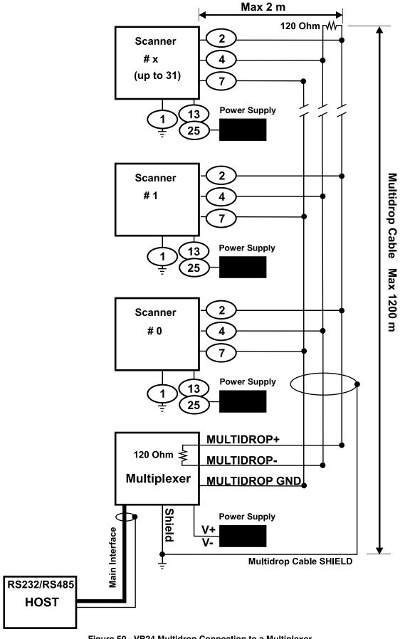
Figure 50 - VB24 Multidrop Connection to a Multiplexer
