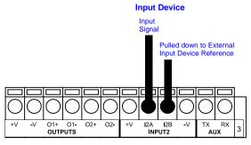
Figure 37 - PNP Input 2 Using External Power
