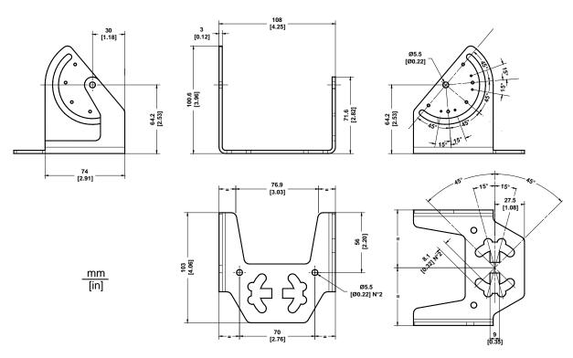
Figure 14 – U Shape Mounting Bracket Overall Dimensions
