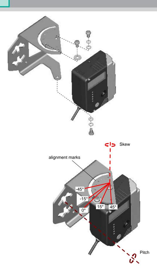
Figure 16 – Positioning with U Shape Mounting Bracket
