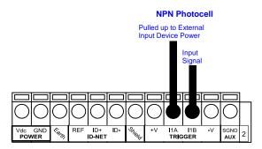
Figure 36 - NPN External Trigger Using External Power
