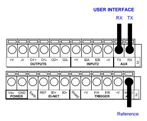
Figure 32 - RS232 Auxiliary Interface Connections
