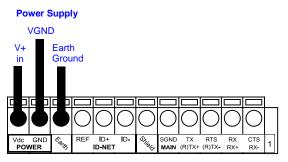
**Figure 20 - Power Supply Connections**
