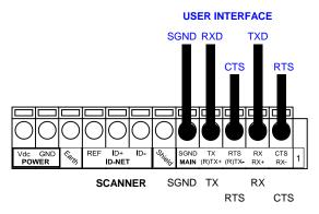
Figure 21 – RS232 Main Interface Connections Using Hardware Handshaking
