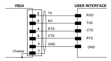
Figure 45 - RS232 Main Interface Connections Using Hardware Handshaking
