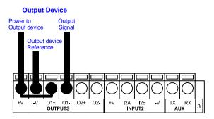
Figure 39 - Open Emitter Output Using VB24 Power
