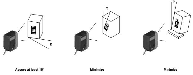
Figure 4 -Skew, Tilt and Pitch Angles
