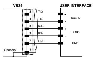
Figure 47 - RS485 Full-duplex Connections
