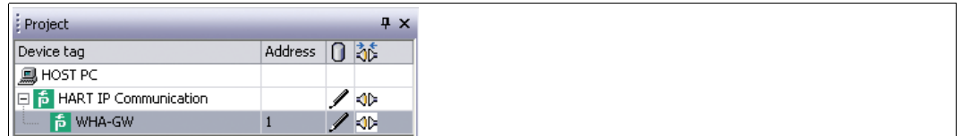
Figure 4.6 New device below HART IP Communication DTM in project tree
