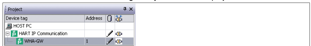
Figure 6.4 New device below HART IP Communication DTM in project tree
