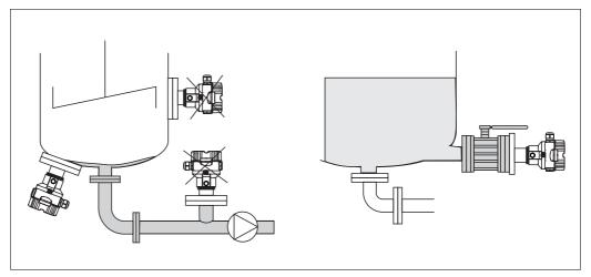
8 Measuring arrangement for level
