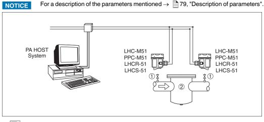
20 Delectrical differential pressure measurement with gauge pressure sensors
