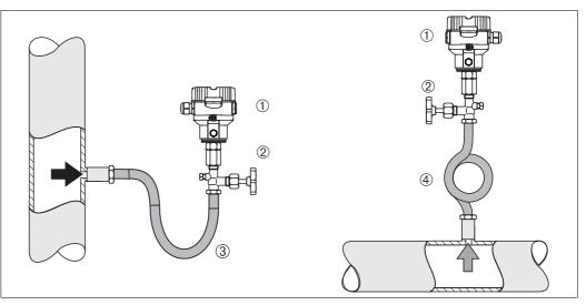
Measuring arrangement for pressure measurement in steams 6
