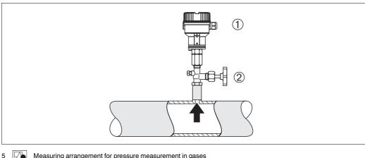
Measuring arrangement for pressure measurement in gases
