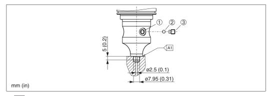
11 🕢 Version XSJ: prepared for diaphragm seal mount
