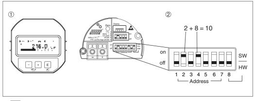
18 🕢 Setting the device address via DIP switches
