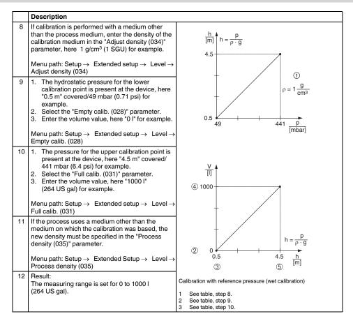
NOTICE The measured variables %, level, volume and mass are available for this level mode see parameter "Unit before lin (025)" in the Operating Instructions.
