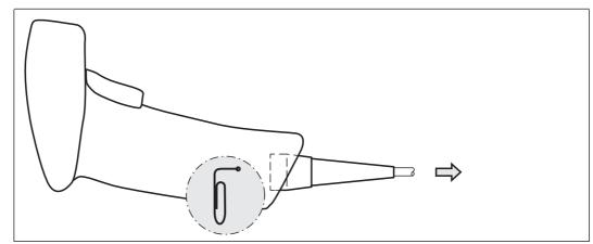
2. Carefully pull the cable complete with RJ50 plug out of the handle.
