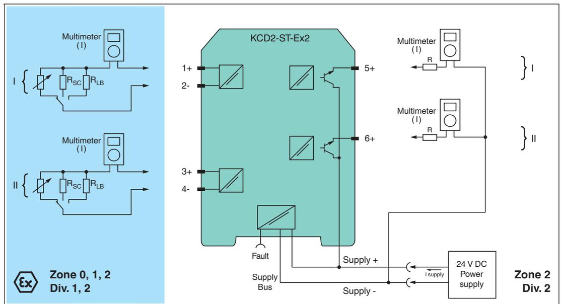
Figure 5.2 Proof test set-up for KCD2-ST-(Ex)2(.SP)
