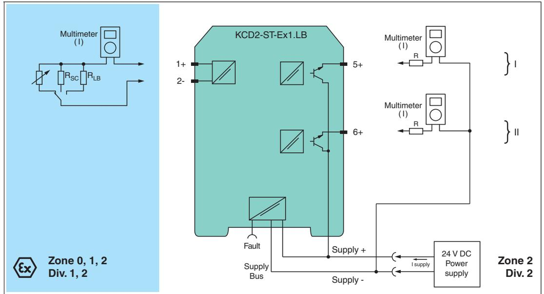
Figure 5.1 Proof test set-up for KCD2-ST-(Ex)1.LB(.SP)
