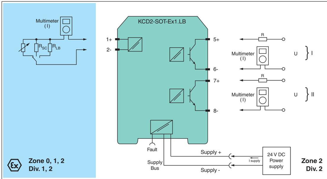
Figure 5.3 Proof test set-up for KCD2-SOT-(Ex)1.LB(.SP)
