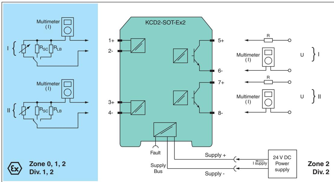
Figure 5.4 Proof test set-up for KCD2-SOT-(Ex)2(.SP)
