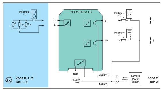
Figure 5.1 Proof test set-up for KCD2-ST-(Ex)1.LB(.SP) Usage in Zone 0, 1, 2/Div. 1, 2 only for Ex versions
