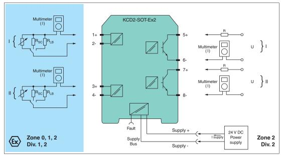
Figure 5.4 Proof test set-up for KCD2-SOT-(Ex)2(.SP) Usage in Zone 0, 1, 2/Div. 1, 2 only for Ex versions
