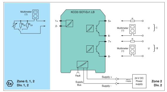
Figure 5.3 Proof test set-up for KCD2-SOT-(Ex)1.LB(.SP) Usage in Zone 0, 1, 2/Div. 1, 2 only for Ex versions
