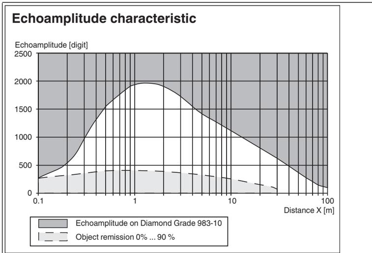
Figure 10.2 Amplitude characteristics OMD30M-R2000-B23-V1V1D\*; OMD30M-R2000-B23-V1VD-HD-1L (ends at 30m); OMD12M-R2000-B23\* (ends at 12 m)
