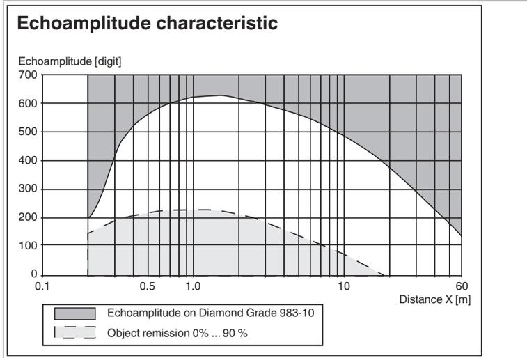
Figure 10.1 Amplitude characteristics for OMD10M-R2000-B23-V1V1D\*
