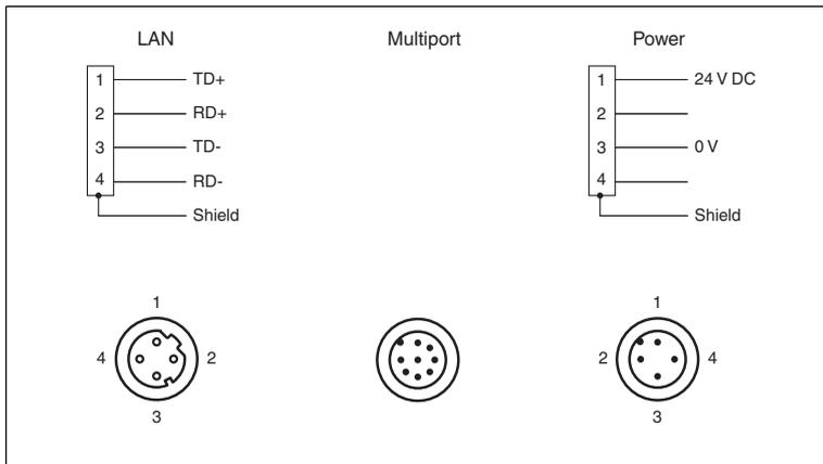
Figure 5.2 R2000 pin assignment
