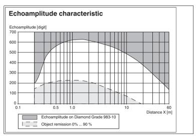
Figure 10.1 Amplitude characteristics for OMD10M-R2000-B23-V1V1D\*
