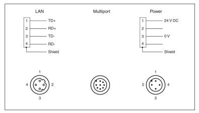
Figure 5.2 R2000 pin assignment
