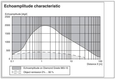
Figure 10.2 Amplitude characteristics OMD30M-R2000-B23-V1V1D\*; OMD30M-R2000-B23-V1VD-HD-1L (ends at 30 m); OMD12M-R2000-B23\* (ends at 12 m)
