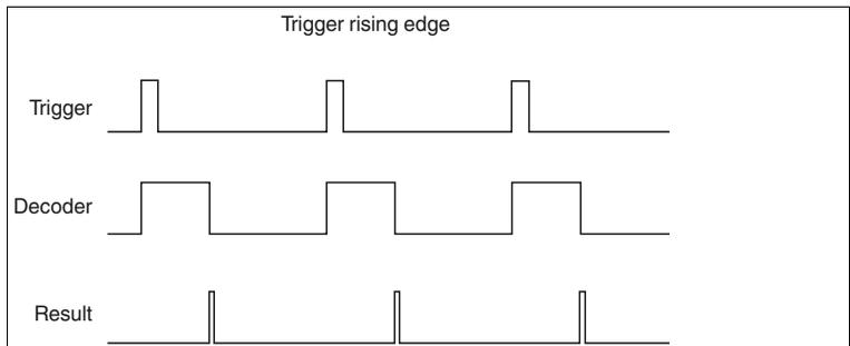
Figure 7.1 Pulse diagram trigger rising edge
