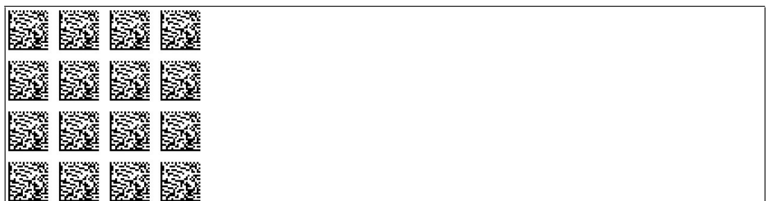
Figure 8.7 The code card assigns the 20 kBaud baud rate to the read head
