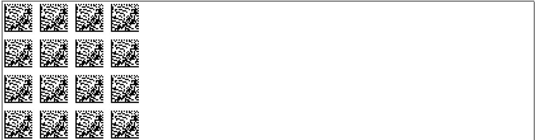
Figure 8.13 The code card assigns the auto baud rate to the read head.
