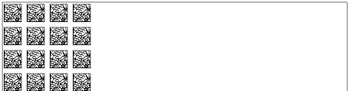
Figure 8.6 The code card assigns the 10 kBaud baud rate to the read head
