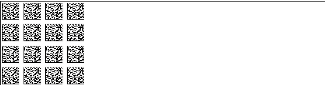
Figure 8.11 The code card assigns the 500 kBaud baud rate to the read head
