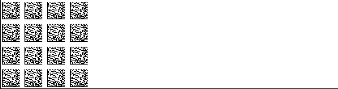
Figure 8.8 The code card assigns the 50 kBaud baud rate to the read head
