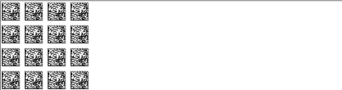
Figure 8.9 The code card assigns the 125 kBaud baud rate to the read head
