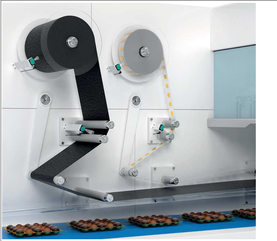
Figure 2.1 Example of application: film monitoring on a packaging machine
