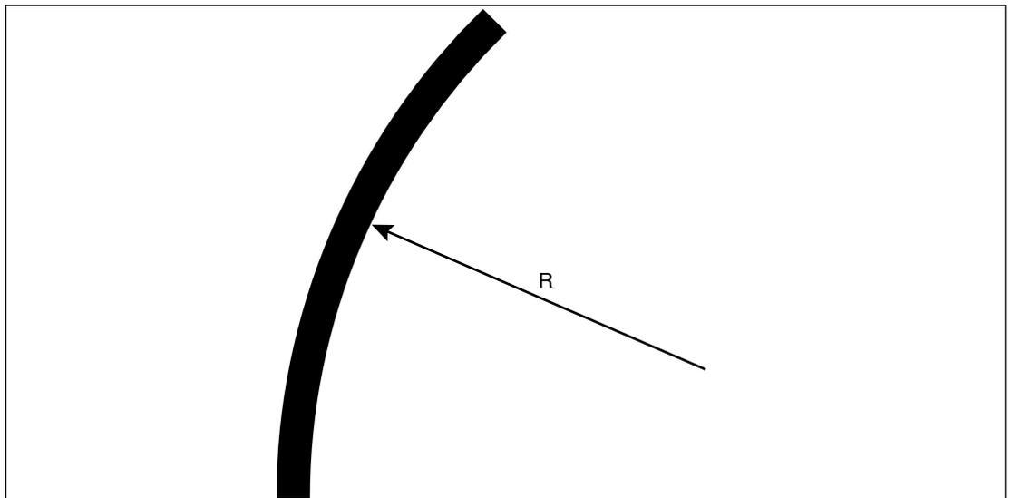
Figure 5.4 Curve radius:  $R \geq 50$  cm
