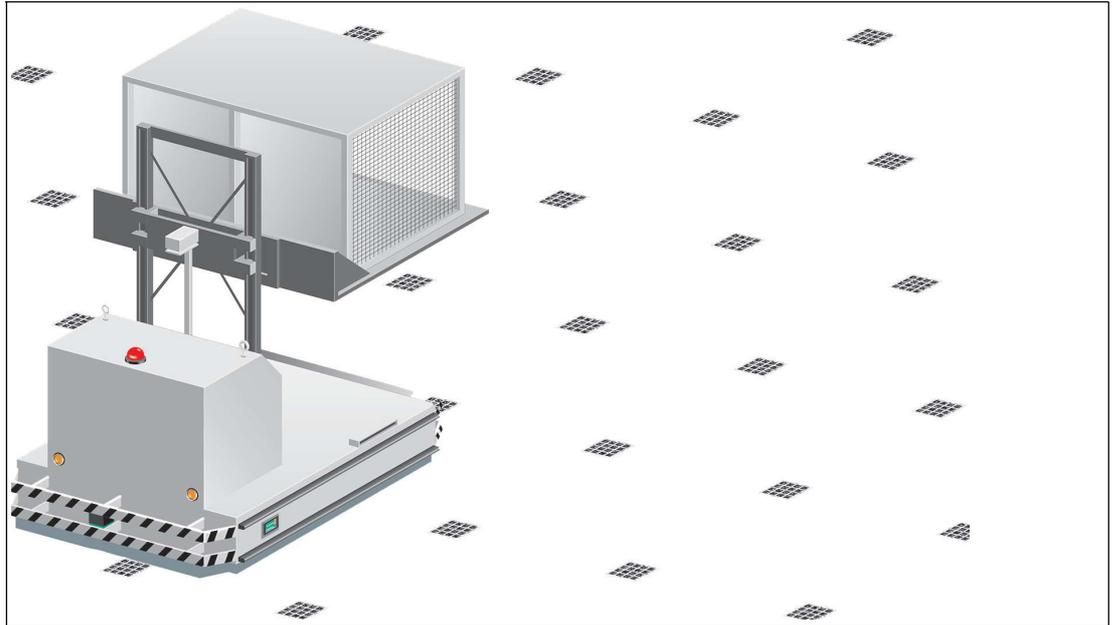
Figure 4.2 Automated guided vehicle with Data Matrix tags
