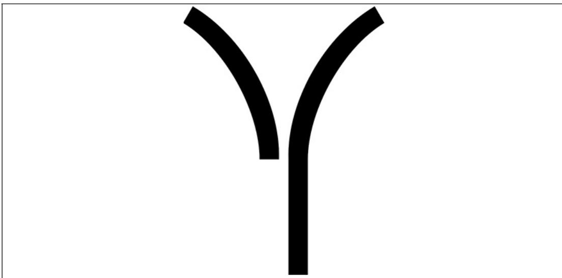
Figure 5.9 Separate lane branches off/converges
