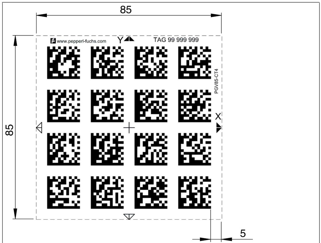
Figure 5.22 Data Matrix tag with the number 99999999 and position information
