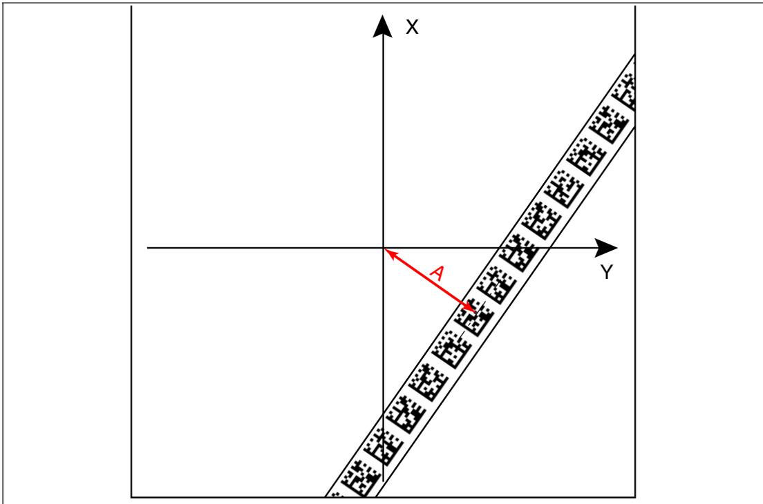
Figure 5.8 Distance A for Data Matrix code tape
