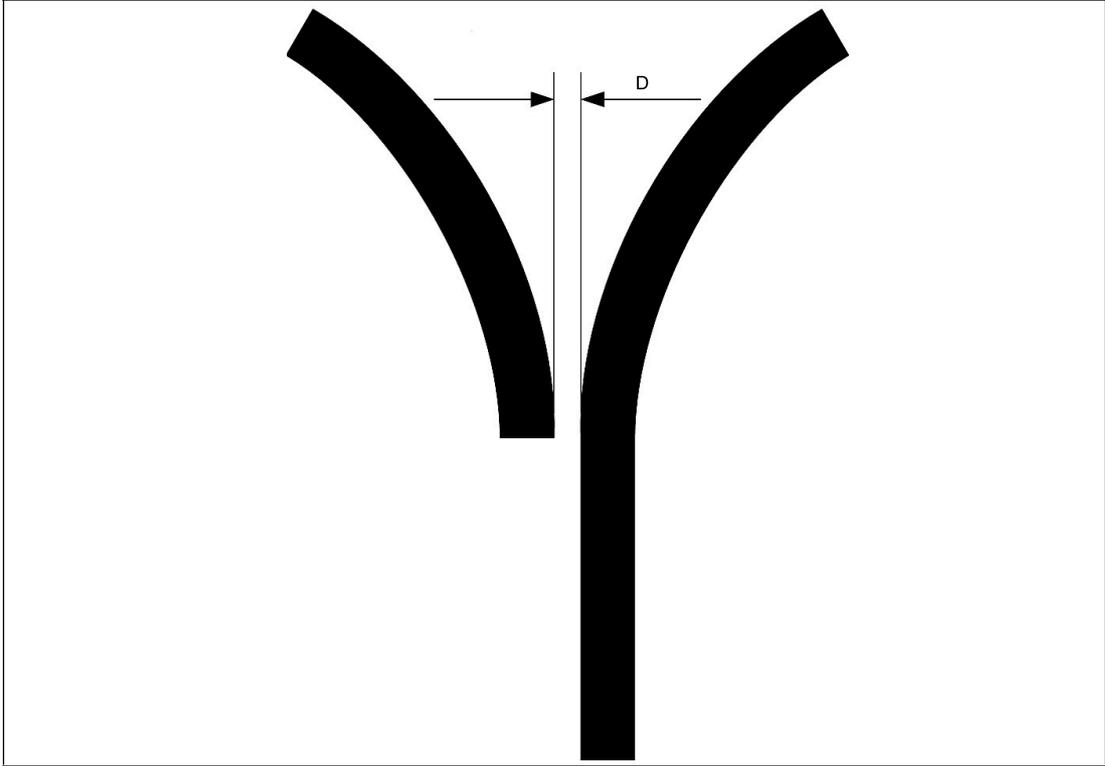
Figure 5.16 Distance:  $7.5 \text{ mm} \leq D \leq 15 \text{ mm}$
