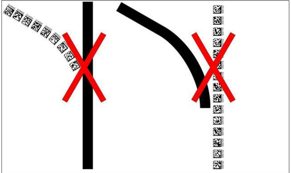
Figure 5.13 Mixture of lanes with colored tape and Data Matrix codes
