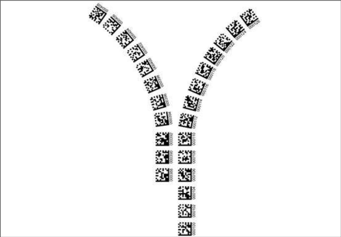
Figure 5.10 Separate lane branches off/converges
