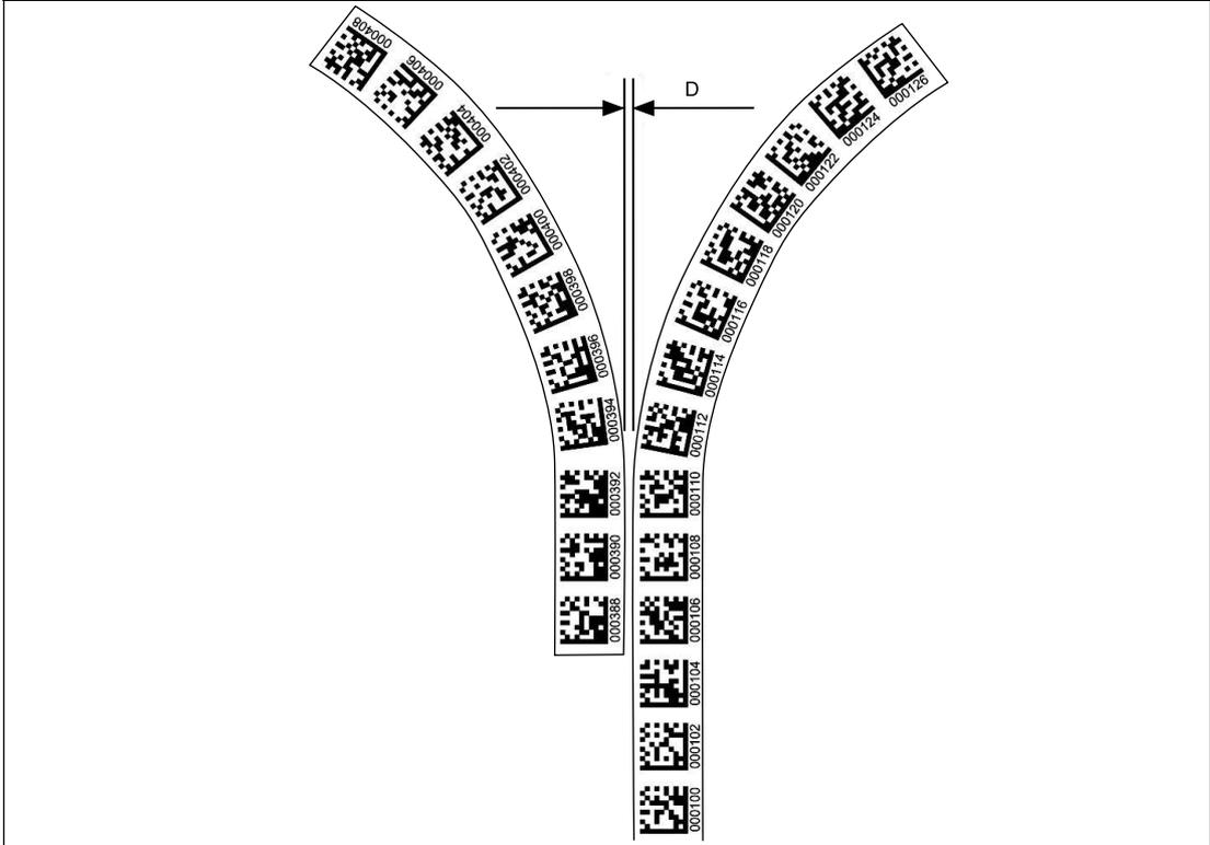
Figure 5.17 Distance:  $0 \text{ mm} \leq D \leq 5 \text{ mm}$
