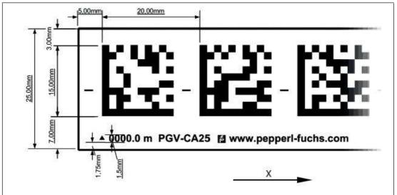
Figure 5.21 The center line indicates the center of the code tape and not the center of the code
