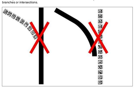
Figure 5.13 Mixture of lanes with colored tape and Data Matrix codes
