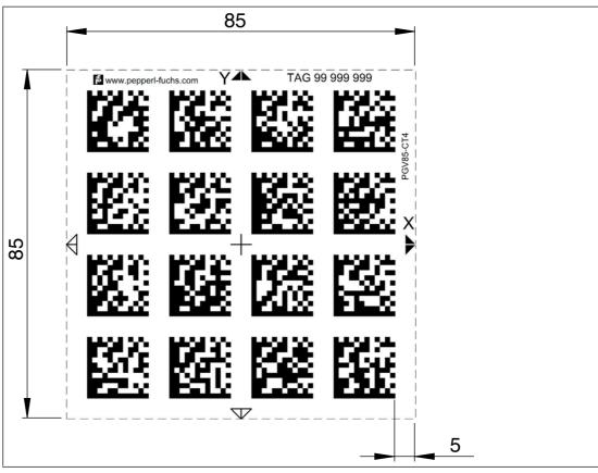
Figure 5.22 Data Matrix tag with the number 99999999 and position information
