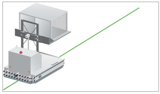
Figure 4.1 Automated guided vehicle with green colored tape
