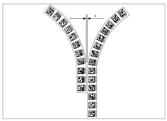
Figure 5.17 Distance:  $0 \text{ mm} \le D \le 5 \text{ mm}$
