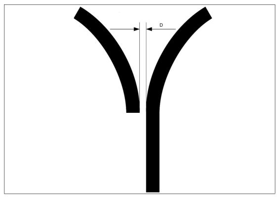
Figure 5.16 Distance: 7.5 mm  $\leq$  D  $\leq$  15 mm
