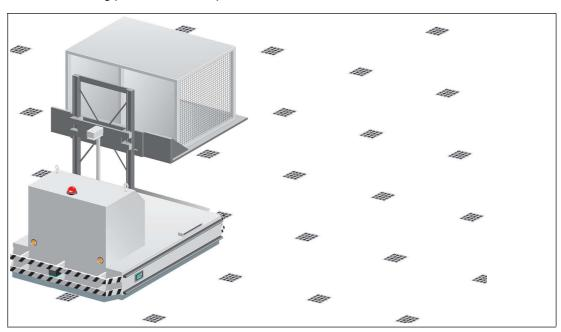
Figure 4.2 Automated guided vehicle with Data Matrix tags
