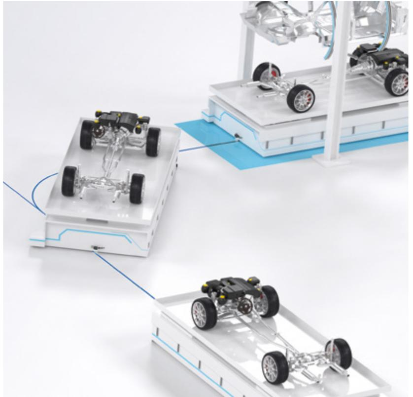
Scanning of the Data Matrix identification/control code initiates the AGV turn.
