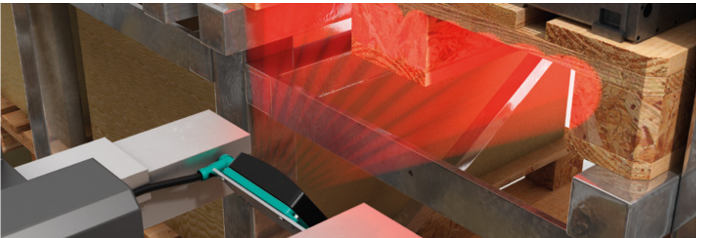
The R2100 detects empty storage bays in an ASRS facility
