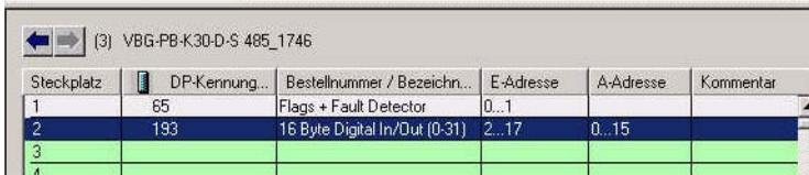
7. Double-clicking on the desired slot line opens a dialog window in which you can assign the PROFIBUS communication module to the address range of the CPU.
