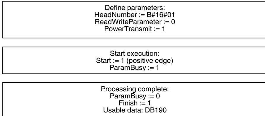
Write: Parameterize three transmission powers
