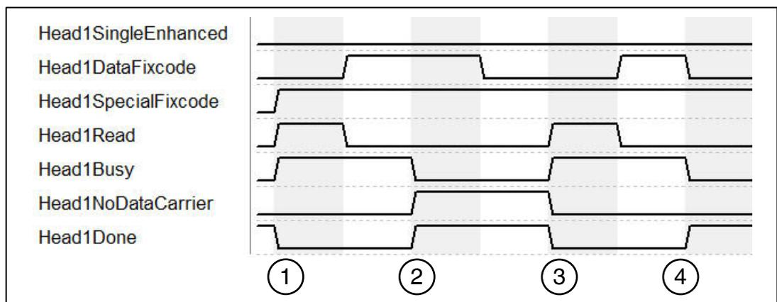
1. "Head1SingleEnhanced" is zero-active in order to initialize a single command. "Head1DataFixcode" is irrelevant as "Head1SpecialFixcode" has higher priority than Words or Fixcode (i.e., as soon as "Head1SpecialFixcode" is TRUE, "Head1DataFixcode" becomes invalid). "Head1DataFixcode" is TRUE in order to access the SpecialFixcode/EPC. Single Read SpecialFixcode is started by "Head1Read" switching to TRUE. "Head1Busy" switches to TRUE; at the same time, "Head1Done" switches to FALSE.
