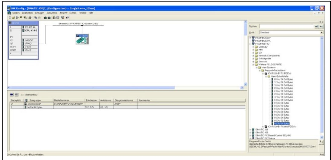
Double-click the IDENTControl icon to open a window containing the properties of the PROFINET node. The name of the PROFINET node (in this case: identcontrol) can be changed in this window if required.
