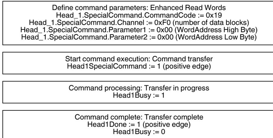
The number of parameterized commands can be increased to a maximum of 10. Parameterization is completed by closing the command list.
