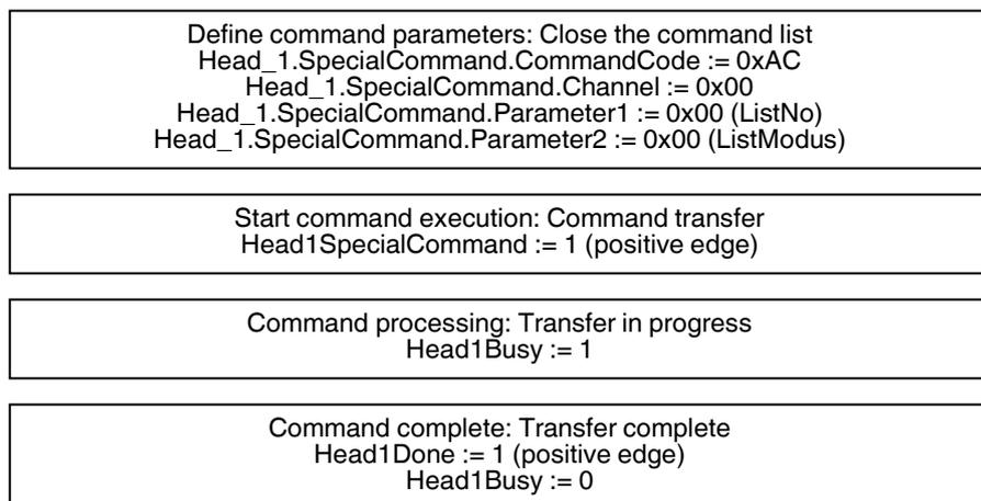
The command list is executed as soon as it is activated. The command list can be activated in single or enhanced mode.
