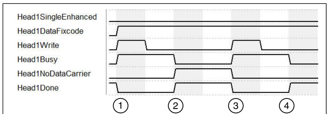
1. "Head1SingleEnhanced" is zero-active in order to initialize a single command. "Head1DataFixcode" is TRUE in order to access the Fixcode/TID. Single Write
