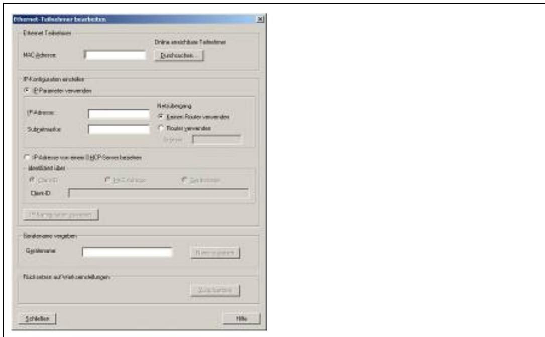
Search for connected nodes in the PROFINET IO system by selecting "Browse...". The IP address and the PROFINET name can then be reassigned.
