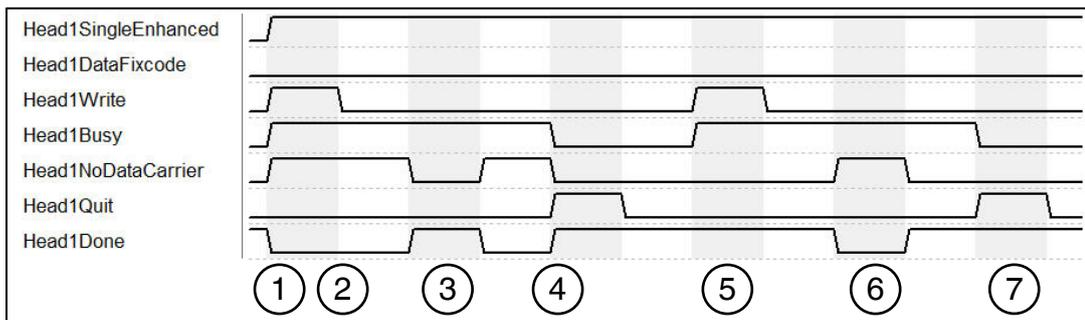
1. "Head1SingleEnhanced" is TRUE in order to initialize an enhanced command. "Head1DataFixcode" is FALSE in order to access Words/User Data. Enhanced Write Words is started, "Head1Write" is TRUE. "Head1Busy" switches to TRUE; at the same time, "Head1Done" switches to FALSE.
