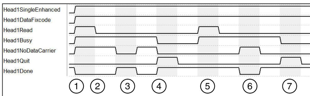
1. Enhanced Read Words is started, "Head1Read" is TRUE. "Head1Busy" switches to TRUE; at the same time, "Head1Done" switches to FALSE.
