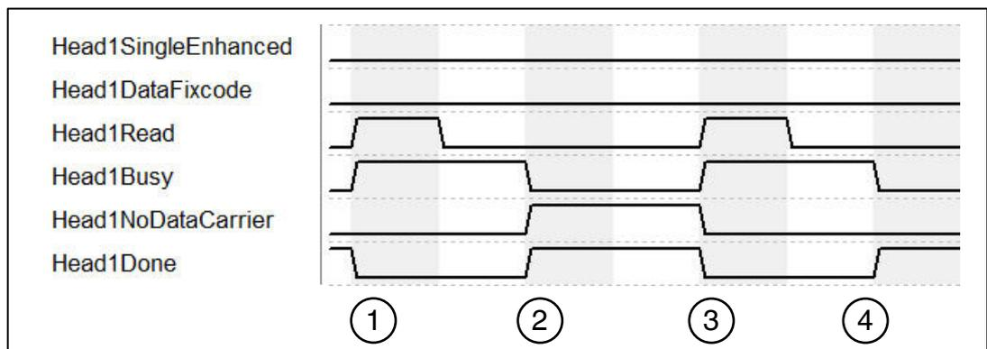
1. "Head1SingleEnhanced" is zero-active in order to initialize a single command. "Head1DataFixcode" is FALSE in order to access words/user data. Single Read Words is started by "Head1Read" switching to TRUE. "Head1Busy" switches to TRUE; at the same time, "Head1Done" switches to FALSE.
