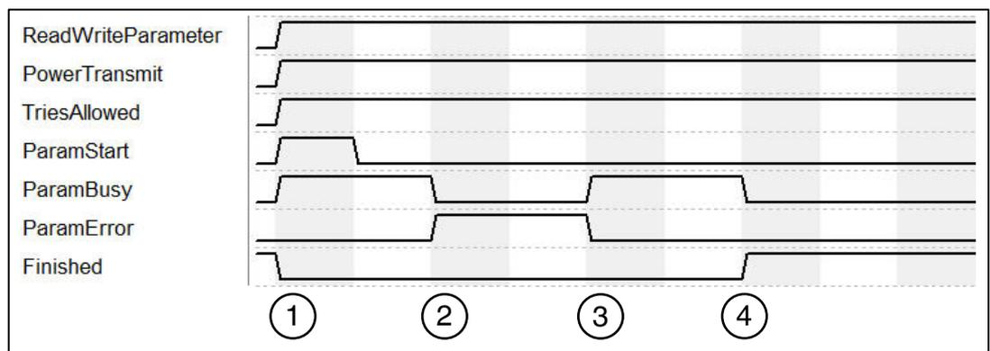
1. Command execution (write) is started with "ParamStart". "ParamFinished" switches to FALSE.
