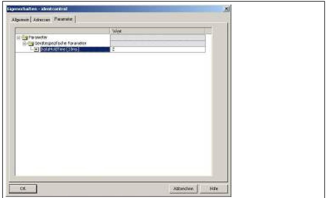
The device-specific parameter "DataHoldTime" (DHT) describes the data hold time within the output data field of the IDENTControl. The DHT should be twice the value of the cycle time of the controller.
