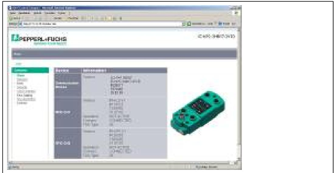
The communication parameters and the PROFINET name can be parameterized by selecting "Network".
