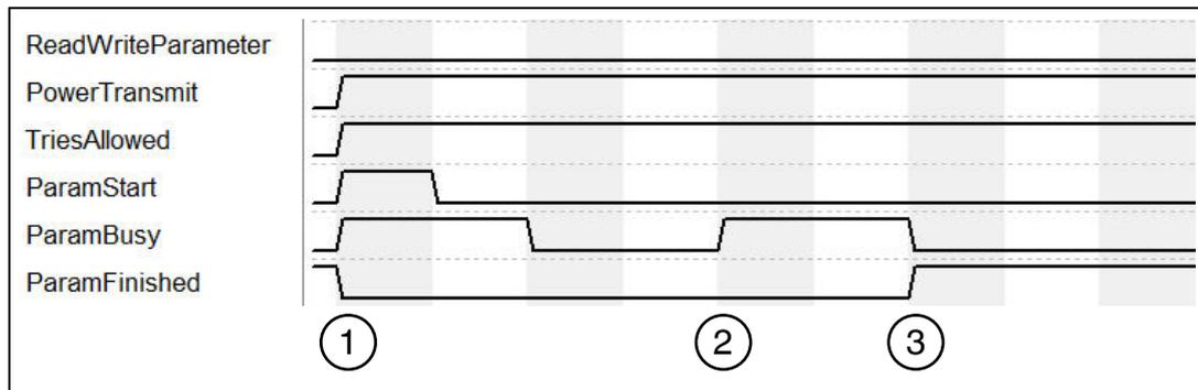
1. Command execution (read) is started with "ParamStart". "ParamFinished" switches to FALSE.
