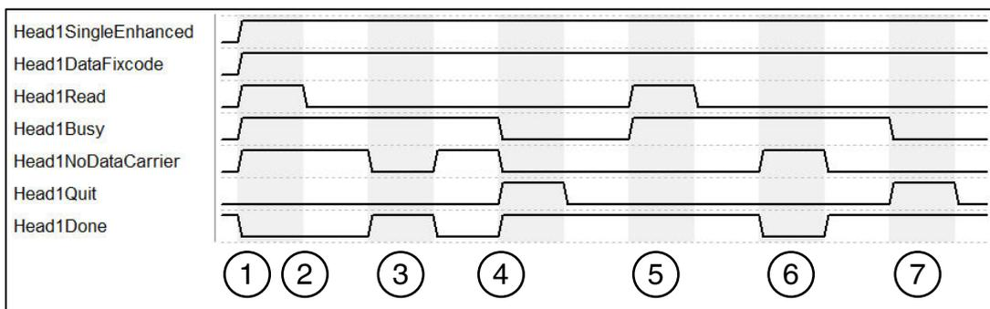
1. "Head1SingleEnhanced" is TRUE in order to initialize an enhanced command. "Head1DataFixcode" is TRUE in order to access the Fixcode/TID. Enhanced Read Fixcode is started, "Head1Read" is TRUE. "Head1Busy" switches to TRUE; at the same time, "Head1Done" switches to FALSE.
