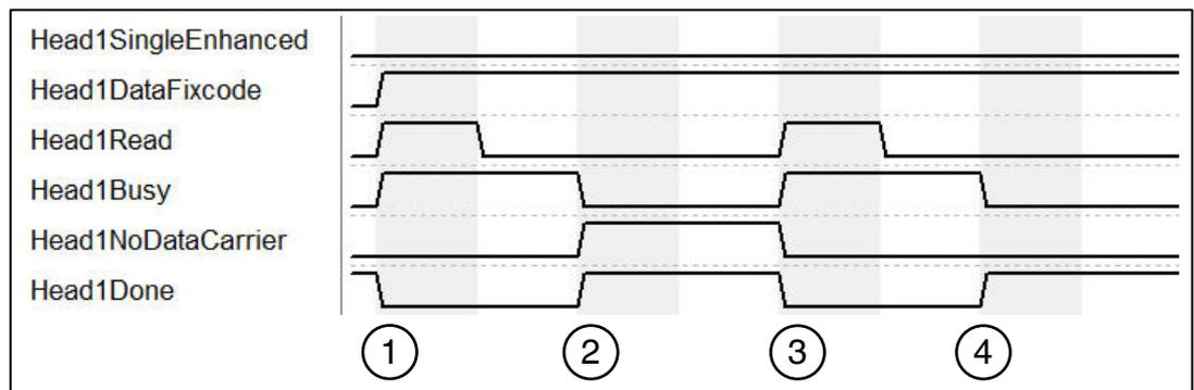
1. "Head1SingleEnhanced" is zero-active in order to initialize a single command. "Head1DataFixcode" is TRUE in order to access the Fixcode/TID. Single Read Fixcode is started by "Head1Read" switching to TRUE. "Head1Busy" switches to TRUE; at the same time, "Head1Done" switches to FALSE.
