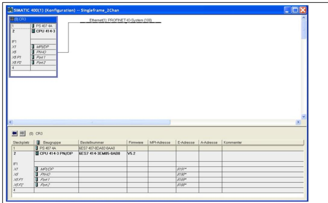
IDENTControl is then connected to the PROFINET IO system In the hardware catalog, select the following and drag to the master system: Additional Field Devices → Ident Systems → Pepperl+Fuchs Ident → "IC-KP2-2HB17 2 PDEV's". The telegram length is then defined by the communication blocks (e.g., In/Out 64 bytes). The module must be assigned to a slot.
