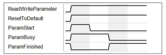
Once the command has been initialized with "ParamStart", "ParamBusy" indicates that command processing is in progress. During this time, "ParamFinished" switches to FALSE. Once the command is complete, "ParamFinished" returns to TRUE.
