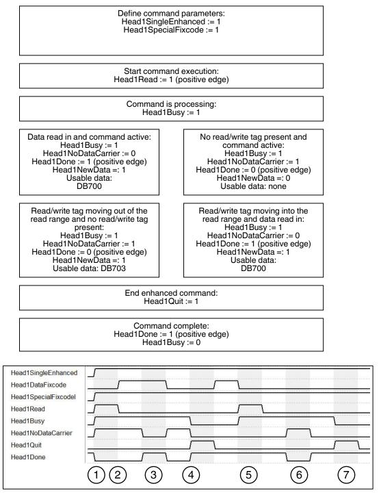
"Head1SingleEnhanced" is TRUE in order to initialize an enhanced command. "Head1DataFixcode" is irrelevant as "Head1SpecialFixcode" has higher priority than Words or Fixcode (i.e., as soon as "Head1SpecialFixcode" is TRUE, "Head1DataFixcode" becomes invalid). "Head1SpecialFixcode" is TRUE in order to access the SpecialFixcode/EPC. Enhanced Read SpecialFixcode is started,
