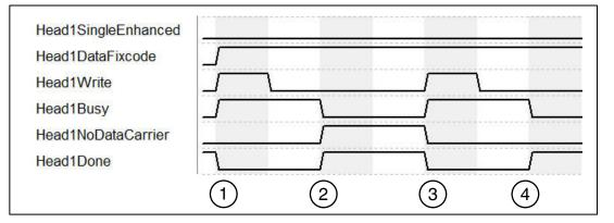
1. "Head1SingleEnhanced" is zero-active in order to initialize a single command. "Head1DataFixcode" is TRUE in order to access the Fixcode/TID. Single Write
