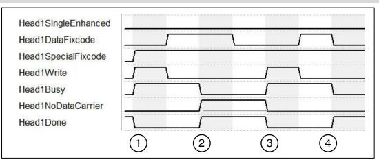
1. "Head1SingleEnhanced" is zero-active in order to initialize a single command. "Head1DataFixcode" is irrelevant as "Head1SpecialFixcode" has higher priority than
