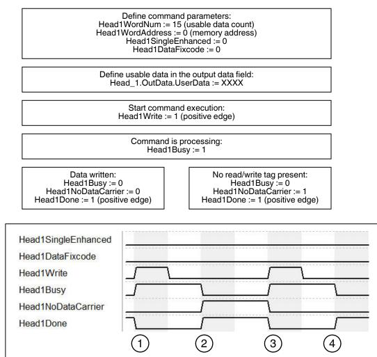
"Head1SingleEnhanced" is zero-active in order to initialize a single command. "Head1DataFixcode" is FALSE in order to access Words/User Data. Single Write Words is started by "Head1Write" switching to TRUE. "Head1Busy" switches to TRUE; at the same time, "Head1Done" switches to FALSE.
