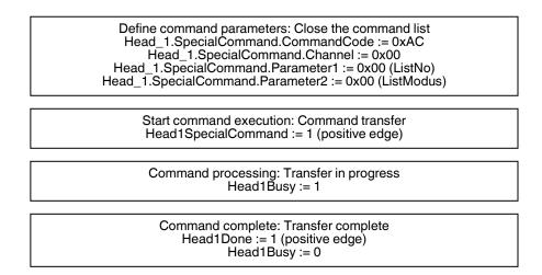
The command list is executed as soon as it is activated. The command list can be activated in single or enhanced mode.
