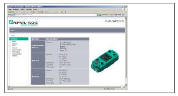
The communication parameters and the PROFINET name can be parameterized by selecting "Network".
