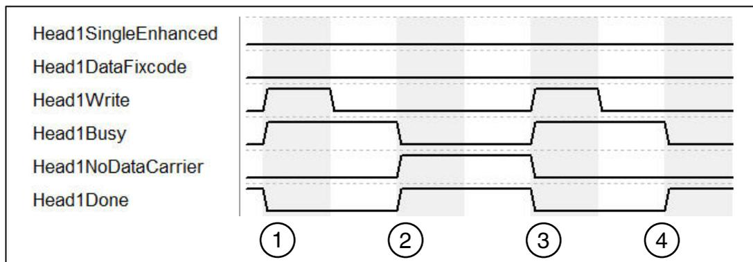
1. "Head1SingleEnhanced" is zero-active in order to initialize a single command. "Head1DataFixcode" is FALSE in order to access Words/User Data. Single Write
