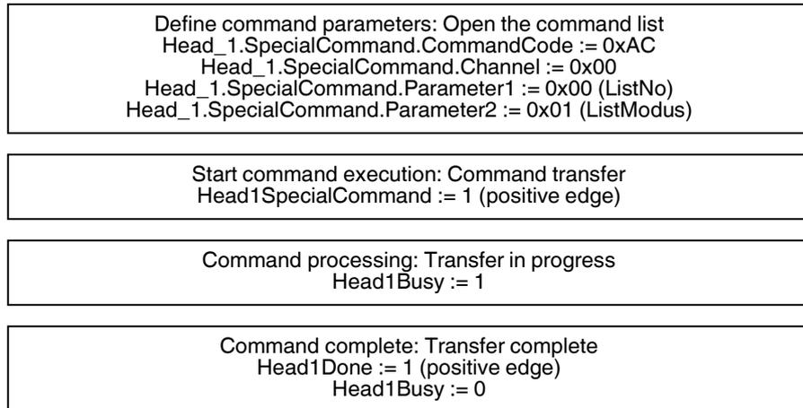
After opening the command list, the commands to be executed are transferred to the control interface by the special command. The Enhanced Read Fixcode command is then parameterized, followed by the Enhanced Read Words command.
