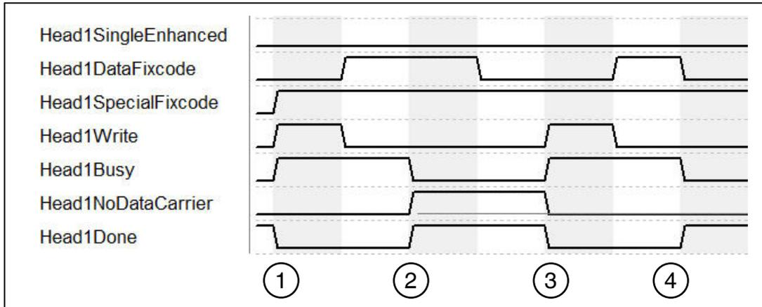
1. "Head1SingleEnhanced" is zero-active in order to initialize a single command. "Head1DataFixcode" is irrelevant as "Head1SpecialFixcode" has higher priority than Words or Fixcode (i.e., as soon as "Head1SpecialFixcode" is TRUE, "Head1DataFixcode" becomes invalid). "Head1DataFixcode" is TRUE in order to access the SpecialFixcode/EPC. Single Write SpecialFixcode is started by "Head1Write" switching to TRUE. "Head1Busy" switches to TRUE; at the same time, "Head1Done" switches to FALSE.
