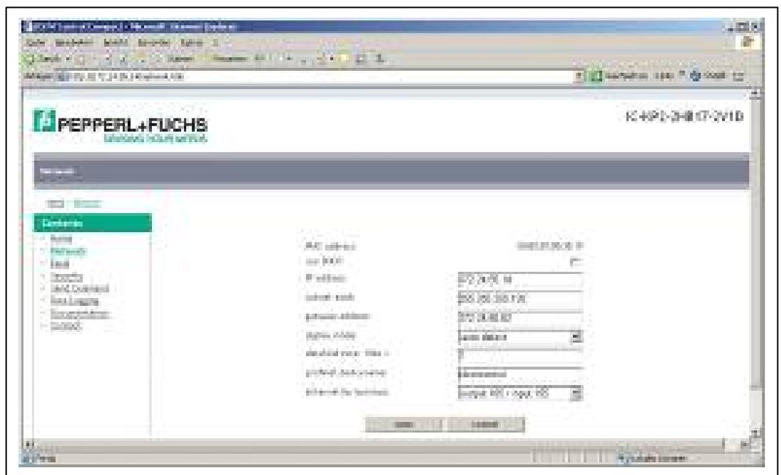
The parameters are applied to the device by selecting "Save". The device will then restart automatically. The new configuration will be activated as soon as the rotary switch on the back of the device is set to the "0" position.
