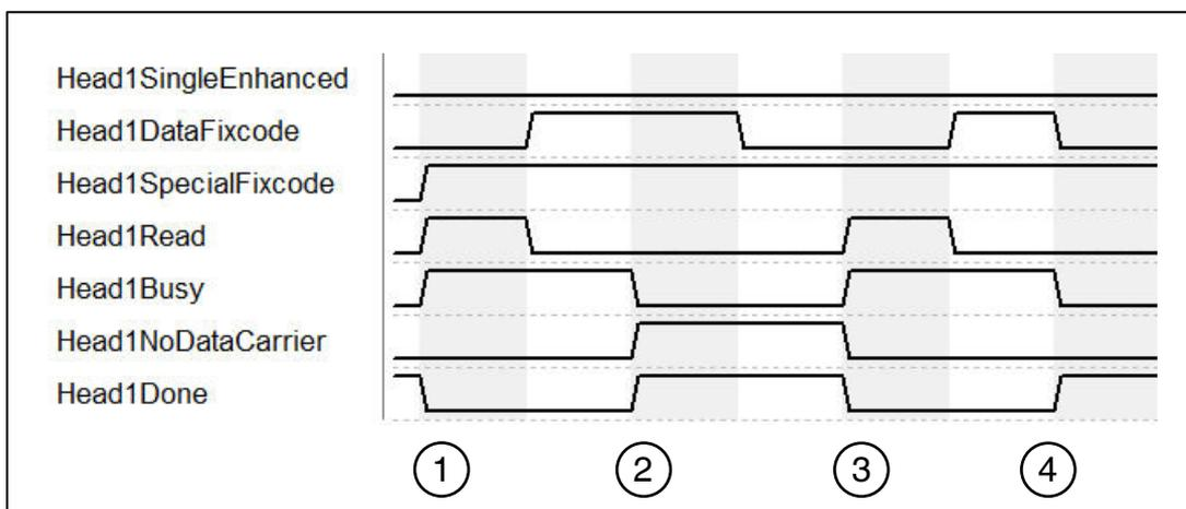
1. "Head1SingleEnhanced" is zero-active in order to initialize a single command. "Head1DataFixcode" is irrelevant as "Head1SpecialFixcode" has higher priority than Words or Fixcode (i.e., as soon as "Head1SpecialFixcode" is TRUE, "Head1DataFixcode" becomes invalid). "Head1DataFixcode" is TRUE in order to access the SpecialFixcode/EPC. Single Read SpecialFixcode is started by "Head1Read" switching to TRUE. "Head1Busy" switches to TRUE; at the same time, "Head1Done" switches to FALSE.
