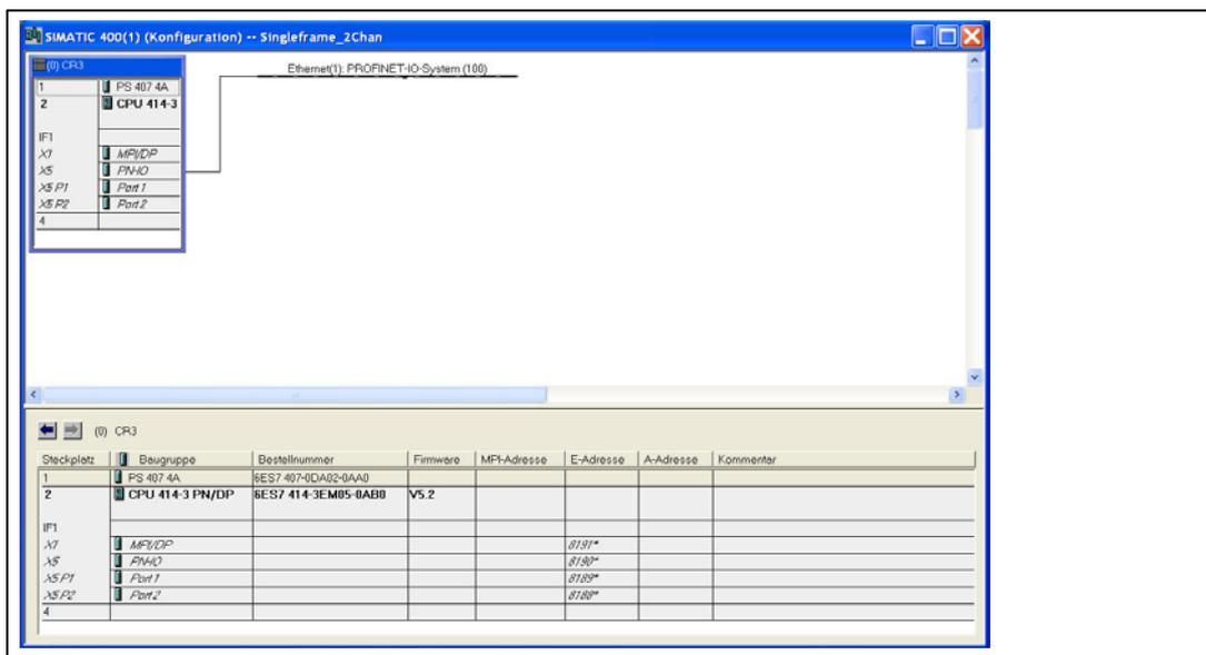
IDENTControl is then connected to the PROFINET IO system In the hardware catalog, select the following and drag to the master system: Additional Field Devices → Ident Systems → Pepperl+Fuchs Ident → "IC-KP2-2HB17 2 PDEV's". The telegram length is then defined by the communication blocks (e.g., In/Out 64 bytes). The module must be assigned to a slot.
