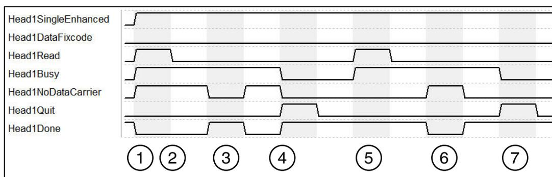
1. "Head1SingleEnhanced" is TRUE in order to initialize an enhanced command. "Head1DataFixcode" is FALSE in order to access words/user data. Enhanced Read Words is started, "Head1Read" is TRUE. "Head1Busy" switches to TRUE; at the same time, "Head1Done" switches to FALSE.
