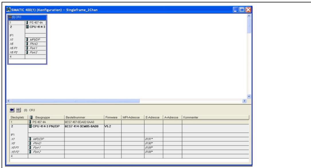
Add a PROFINET IO system by right-clicking on the PROFINET port.
