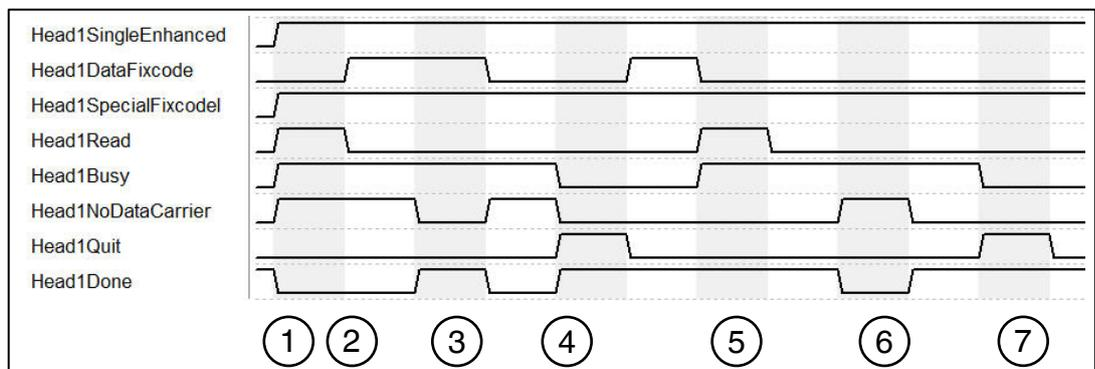
1. "Head1SingleEnhanced" is TRUE in order to initialize an enhanced command. "Head1DataFixcode" is irrelevant as "Head1SpecialFixcode" has higher priority than
