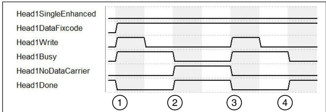
1. "Head1SingleEnhanced" is zero-active in order to initialize a single command. "Head1DataFixcode" is TRUE in order to access the Fixcode/TID. Single Write Fixcode is started by "Head1Write" switching to TRUE. "Head1Busy" switches to TRUE; at the same time, "Head1Done" switches to FALSE.
