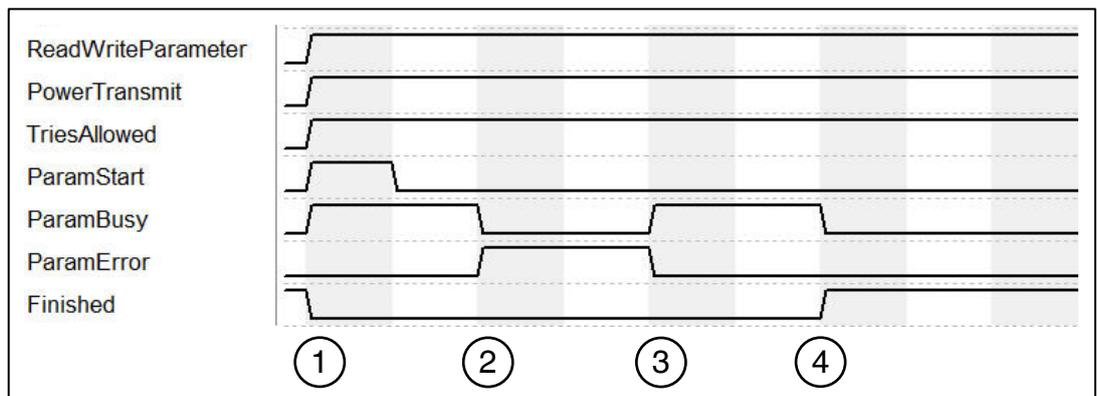
1. Command execution (write) is started with "ParamStart". "ParamFinished" switches to FALSE.
