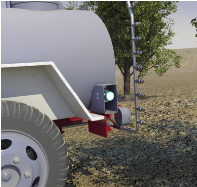
The ultrasonic sensor 30GM70 Series allows direct application of the pesticides.
