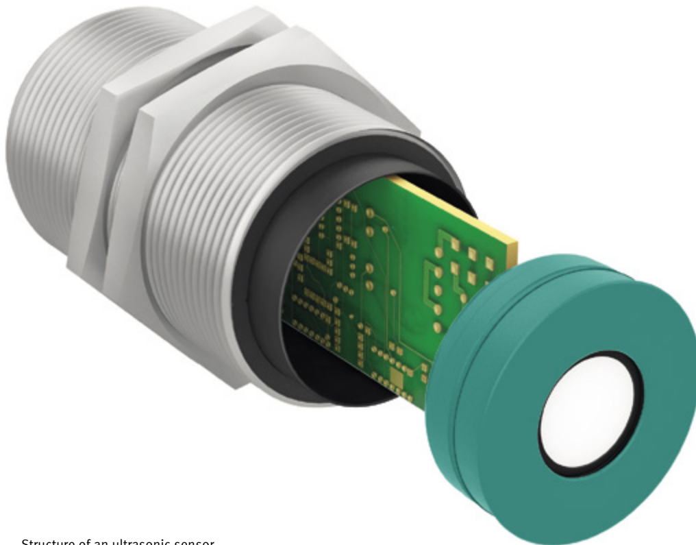
Structure of an ultrasonic sensor.
