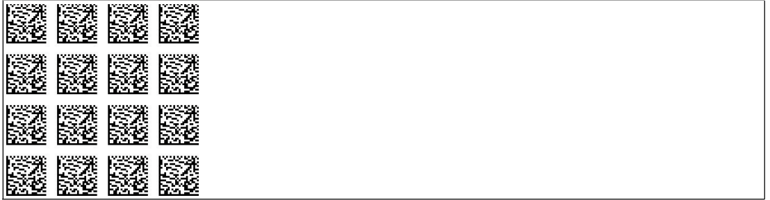
Figure 6.11 The code card assigns the 500 kBaud baud rate to the read head
