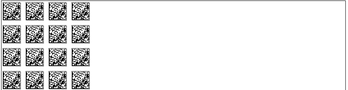
Figure 6.13 The code card assigns the auto baud rate to the read head.
