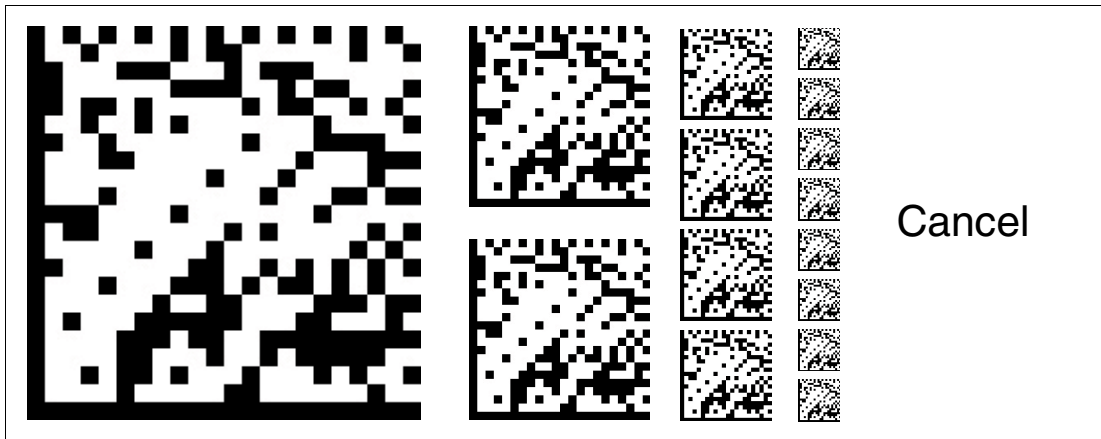
Figure 6.3 The "CANCEL" code card discards the modified parameterization and terminates external parameterization operating mode. The read head switches to normal mode and adopts the last valid configuration that was saved.
