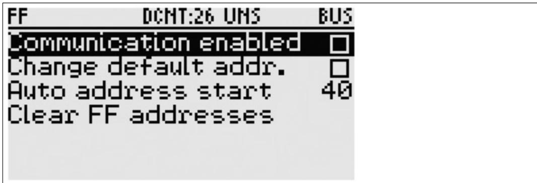
2. "Communication enabled" option: Enables the communication of FDH-1. Communication is required to read device info.
