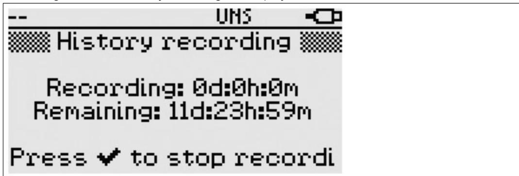
5. In order to interrupt the history recording and store the measures values in a test record: Press the **OK** or **Cancel** key.
