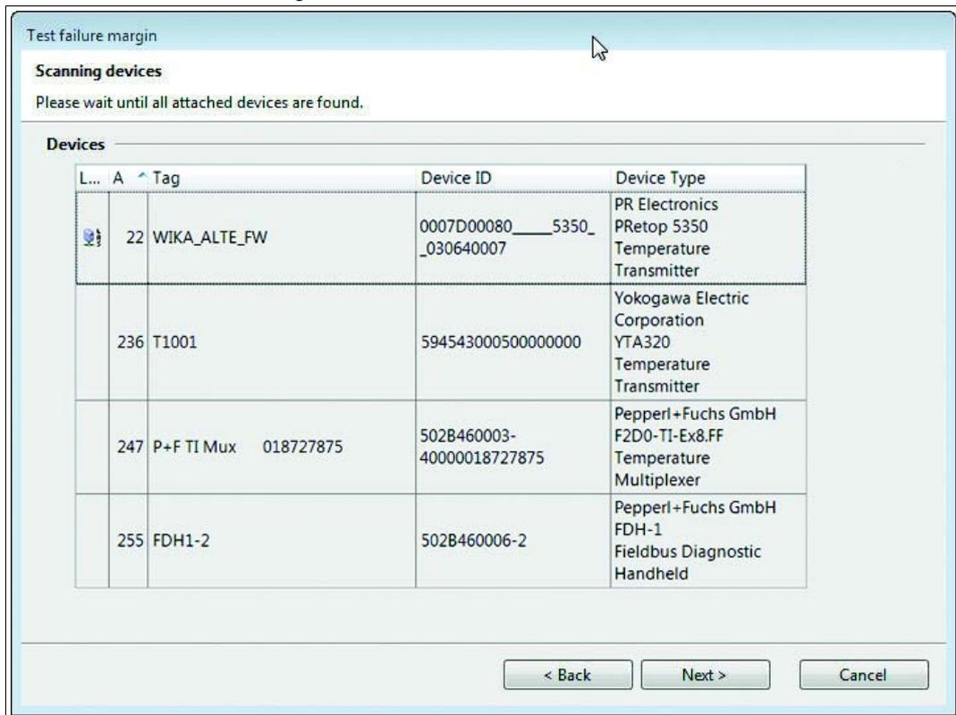
Figure 8.52 FDH-1 Manager: Failure margin test wizard scanning devices
