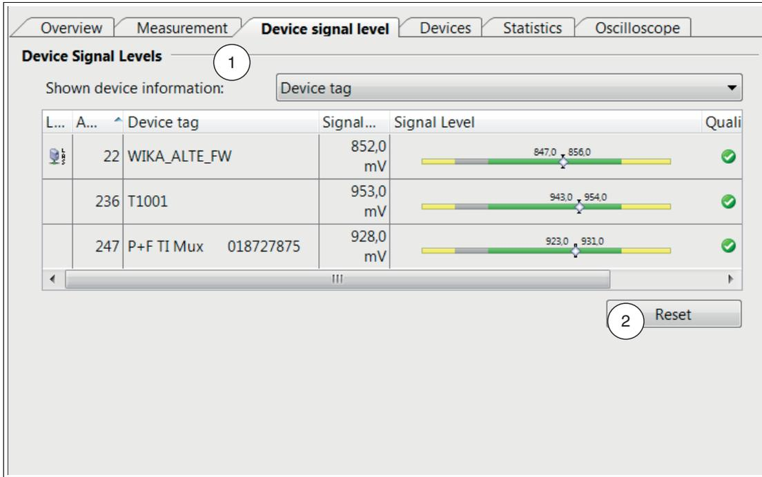
Figure 8.24 FDH-1 device-specific tab: Device signal level
