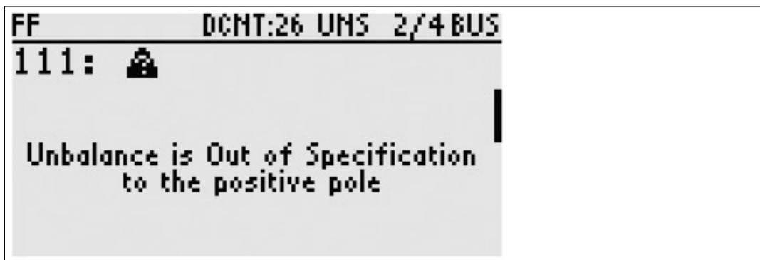
↳ The message screen shows fault indications. Pressing the **Down** arrow key provides possible causes for the fault and suggests resolutions.
