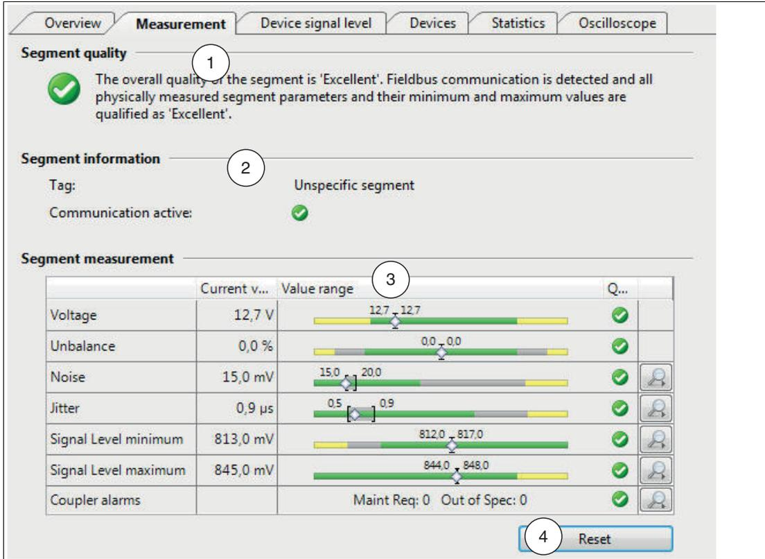
Figure 8.21 FDH-1 device-specific tab: Measurement
