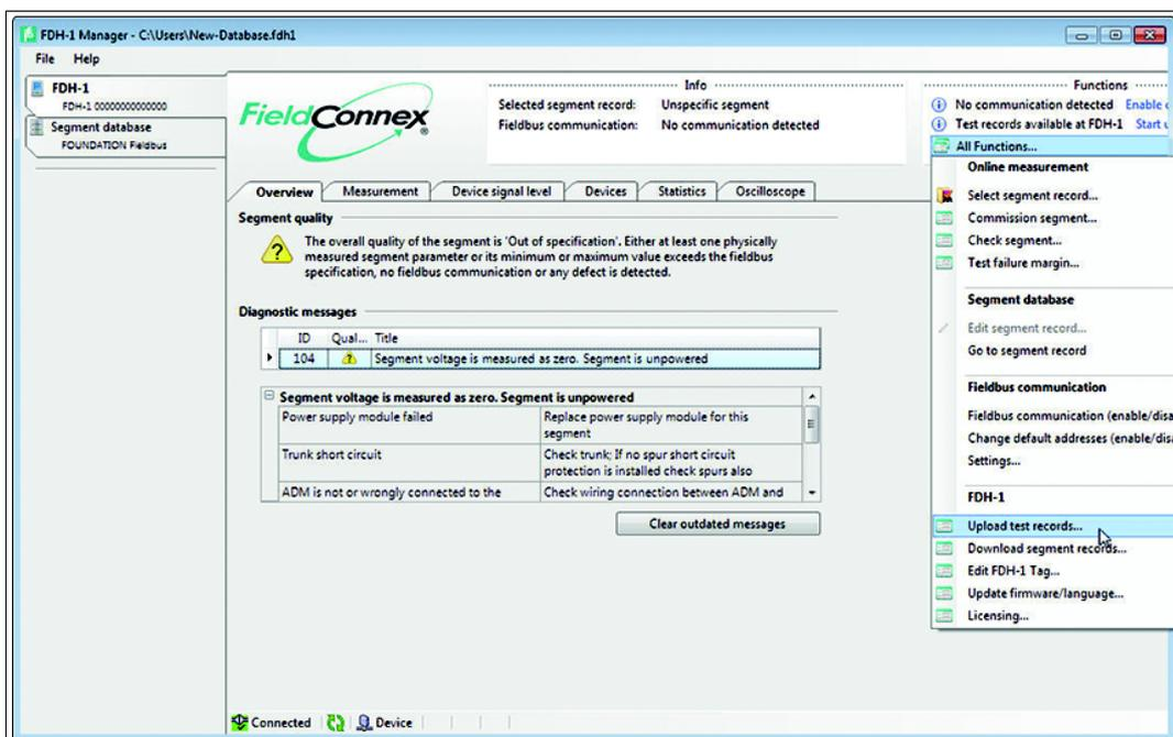
Figure 8.62 FDH-1 Manager Device-specific tab: Go to **All Functions ...** and select **Upload test records**.
