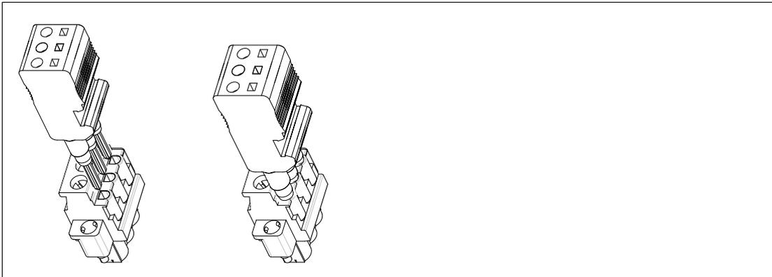
Figure 3.1 Assembly of the test plugs and the fieldbus plug socket
