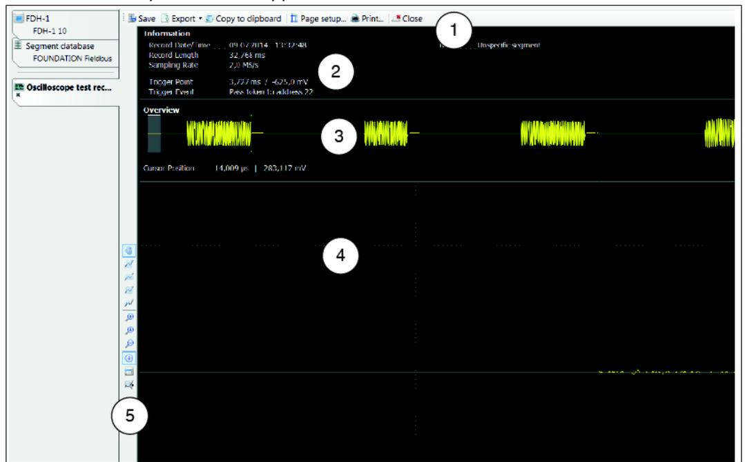
Figure 8.28 FDH-1 Manager device-specific tab: Oscilloscope test record
