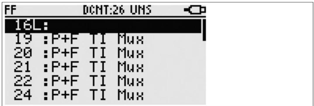
2. In order to select a device, use the **Up** and **Down** arrow keys. In order to start the oscilloscope recording, press the **OK** key.
