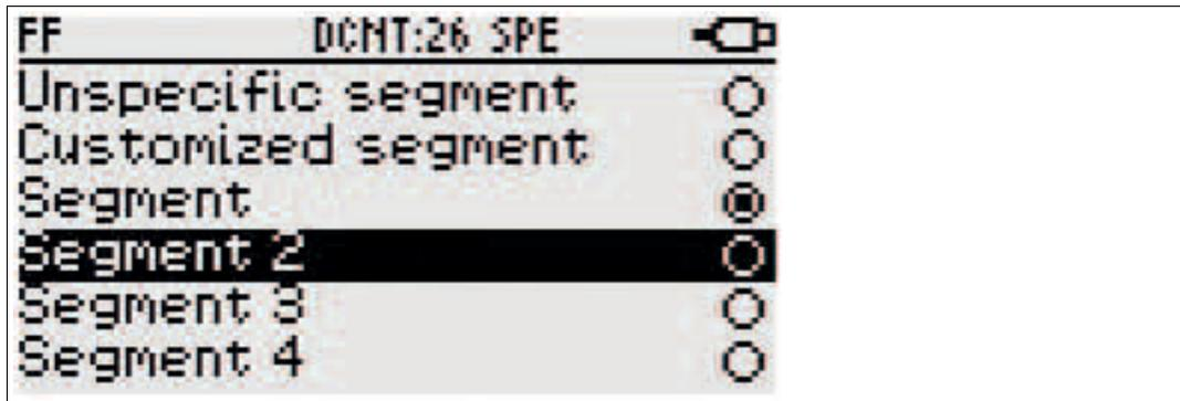
6. FDH-1 asks you to activate the communication function. The communication function is used for actively communicating with the segment devices. In case you want to abort this action and return to the failure margin test menu: press the **Cancel** key. Otherwise, press the **OK** key to proceed.
