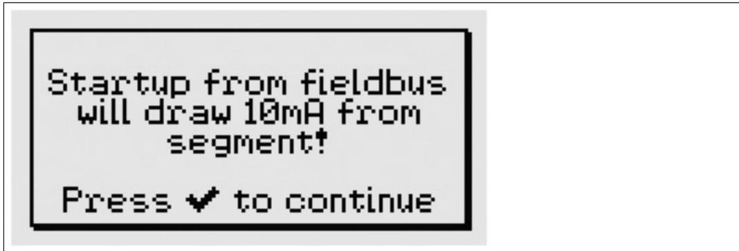
2. In order to confirm, press the **OK** key. The startup screen appears on the LC display:
