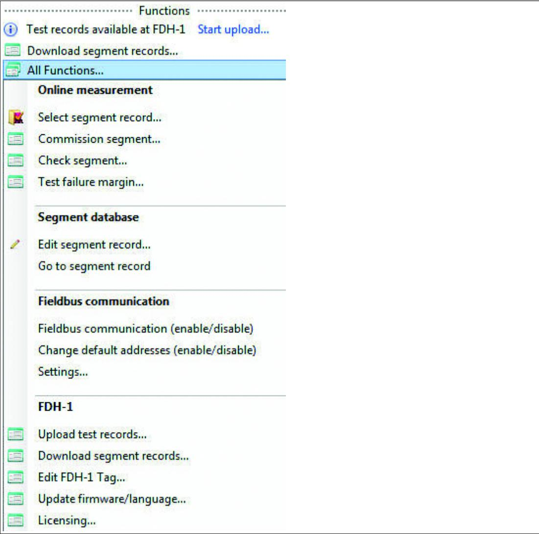
Figure 8.19 The **All Functions...** pulldown menu offers quick access to all tasks and functions that you can carry out with FDH-1 handheld connected to FDH-1 Manager software.
