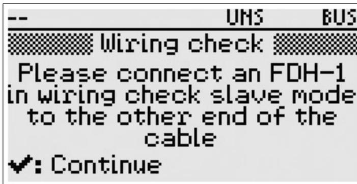
4. Press the **OK** key to launch the test. The test result is displayed on the LC display. If faults are detected, the causes of the faults are issued.
