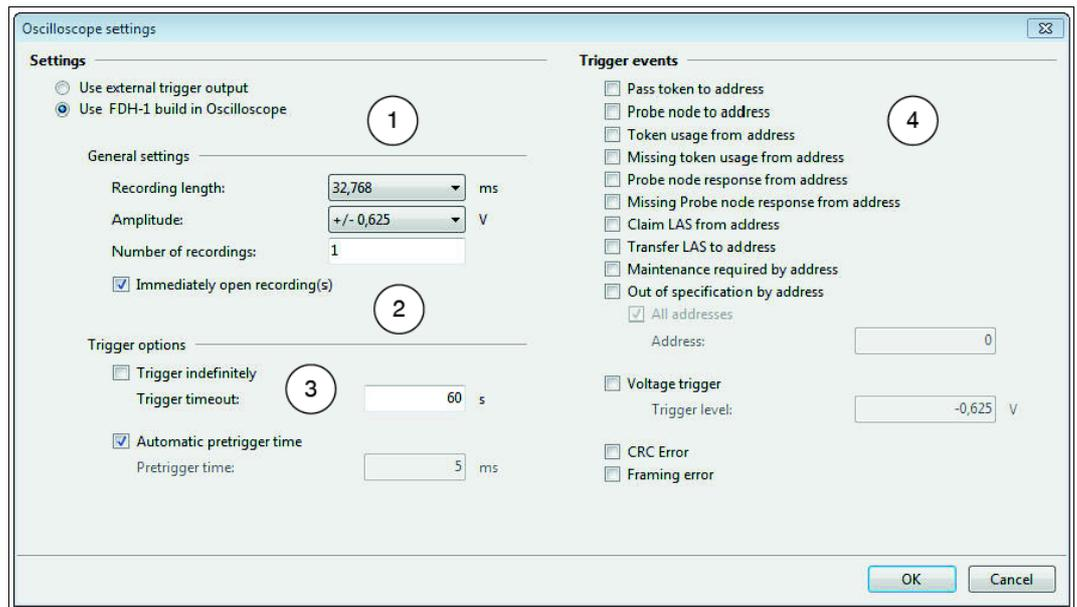
Figure 8.27 FDH-1 Manager device-specific tab: Oscilloscope record settings dialog
