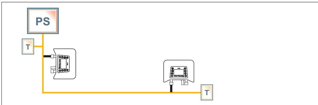
1. Configure the first FDH-1 to run in the “Wiring check master” mode.
