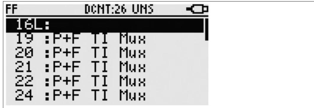
2. In order to select a device, use the **Up** and **Down** arrow keys. In order to start the oscilloscope recording, press the **OK** key.
