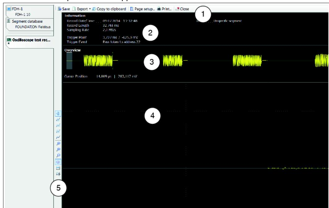
Figure 8.28 FDH-1 Manager device-specific tab: Oscilloscope test record
