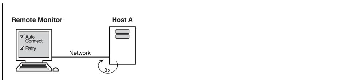
Figure 5.11 Example 3 - Limited number of connection retries to the same host
