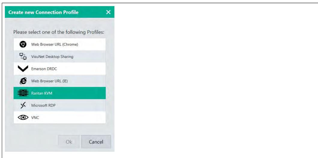
Figure 5.2 The "Create new Connection Profile" dialog box - web browser, Raritan KVM and VisuNet desktop sharing profiles are only available in the pro version.
