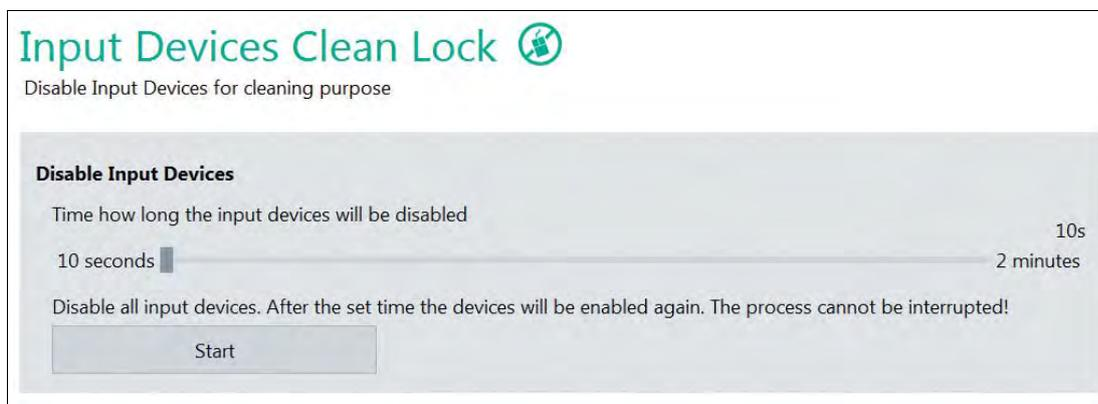
Figure 6.1 System tools - clean lock settings
