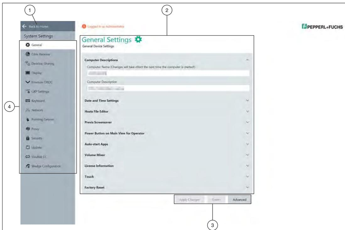
Figure 4.1 Components of the system settings app screen
