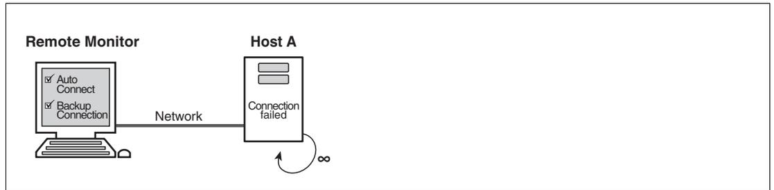
Figure 5.8 Example 1 - Unlimited number of retries to a specific host (with "Backup Connection" feature)
