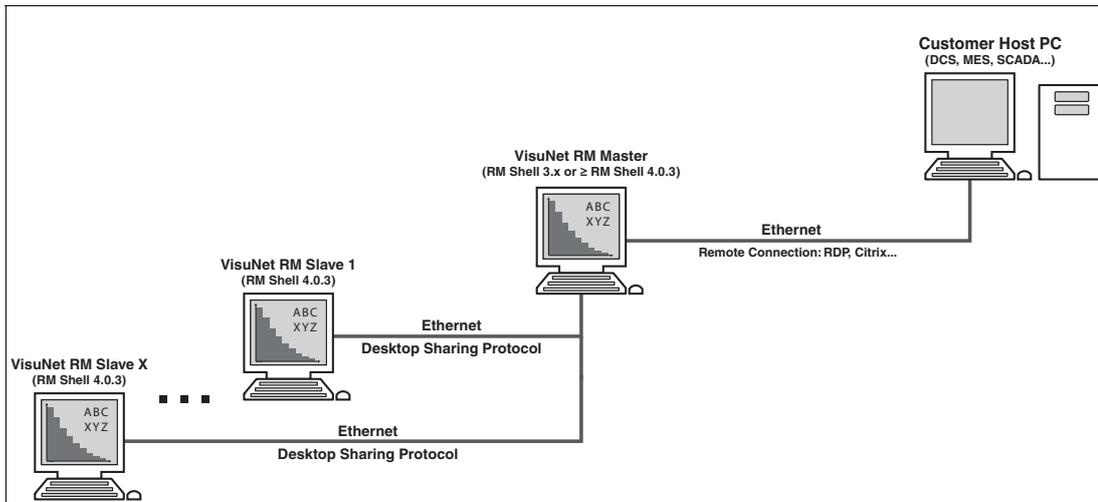
Figure 5.13 Example of a VisuNet desktop sharing infrastructure
