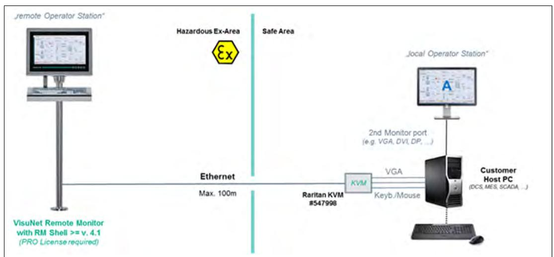
Figure 5.14 Common Setup VisuNet Remote Monitor and Raritan Dominion KVM-o-IP Switch
