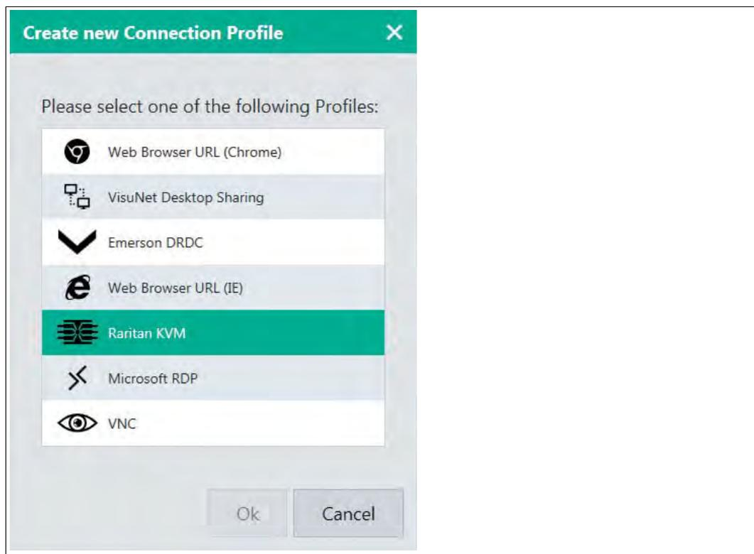
Figure 10.1 The "Create new Connection Profile" dialog box - web browser, Raritan KVM and VisuNet desktop sharing profiles are only available in the pro version.
