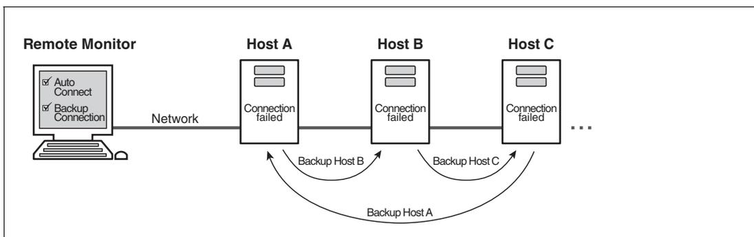
Figure 5.9 Example 2 - unlimited number of connection retries to more than one host (via "Backup Connection" feature)
