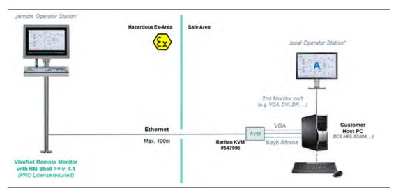
Figure 5.14 Common Setup VisuNet Remote Monitor and Raritan Dominion KVM-o-IP Switch
