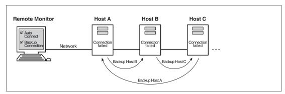
Figure 5.9 Example 2 - unlimited number of connection retries to more than one host (via "Backup Connection" feature)
