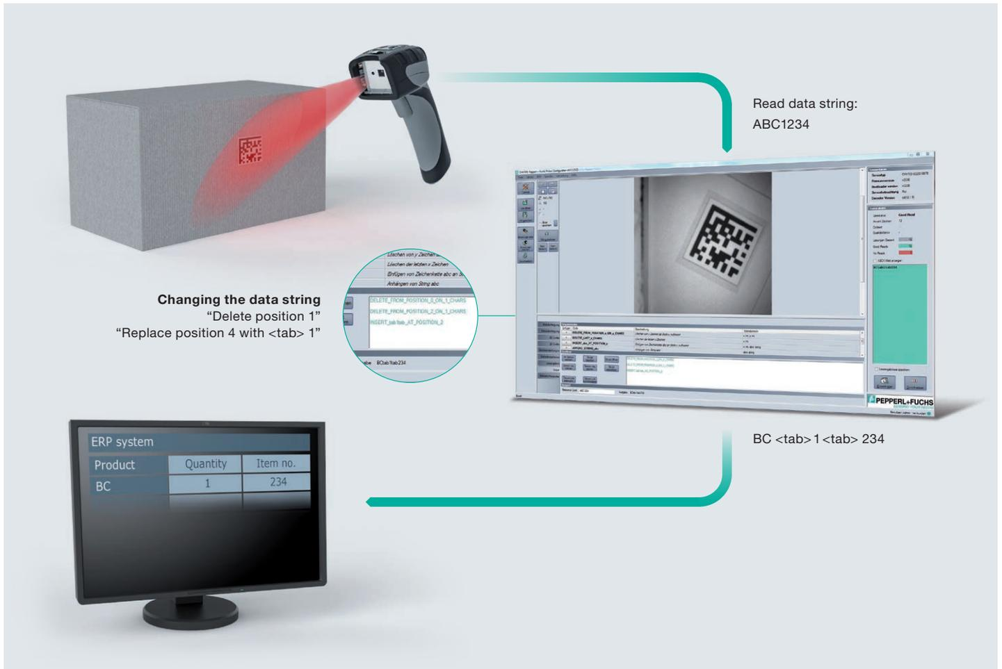
With Pepperl+Fuchs' Vision Configurator, customizing the output string is easy. A read data string can be individually changed and integrated into ERP systems with a simple selection of commands.
