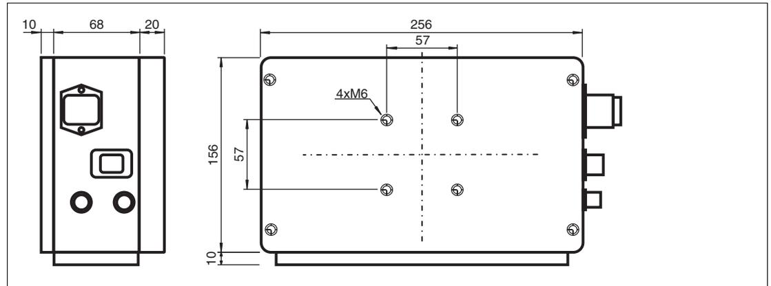
Figure 3.13 Dimensions of the OIT500 system
