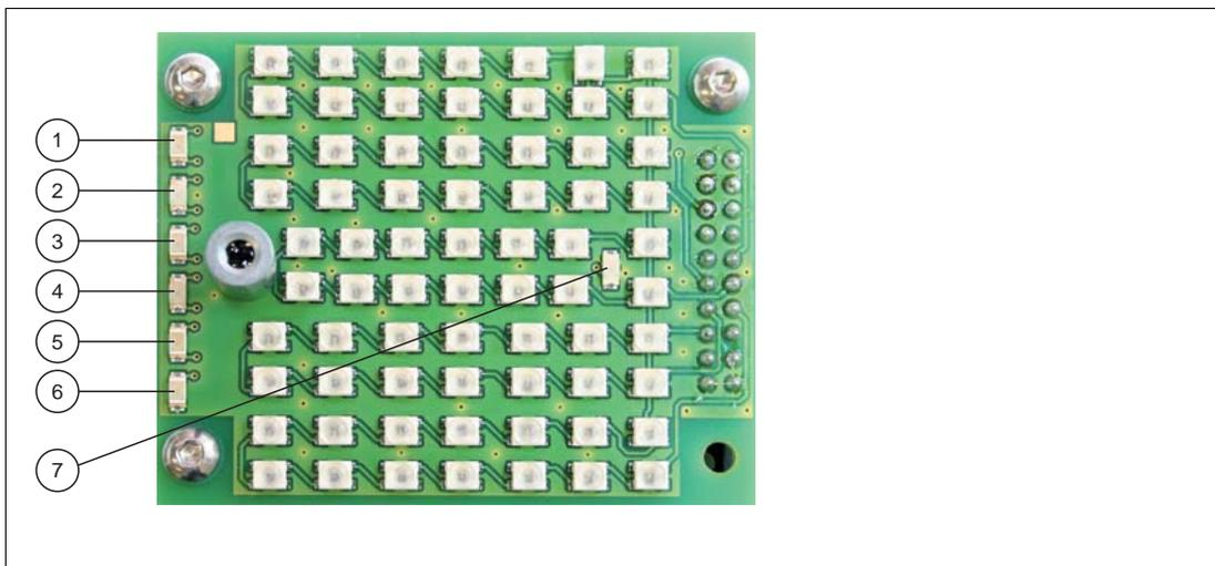
Figure 2.2 Lighting unit of the OIT system
