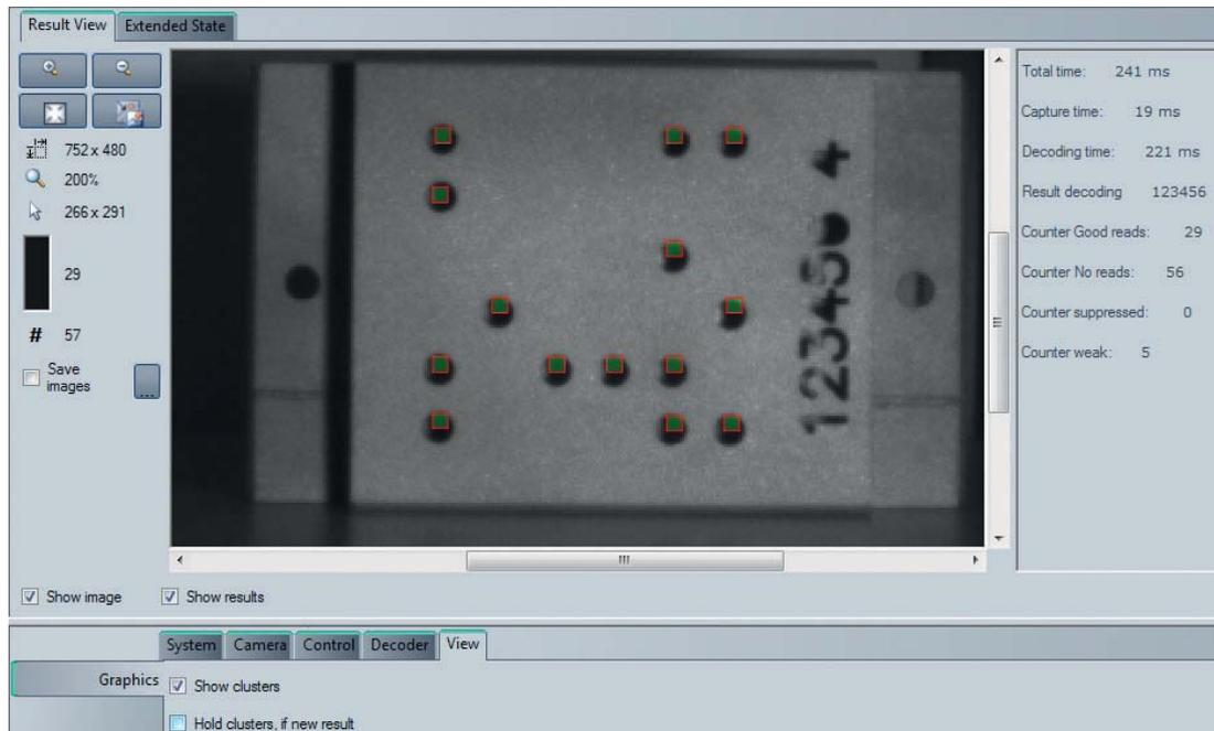
Figure 5.23 Optical marking of the detected holes
