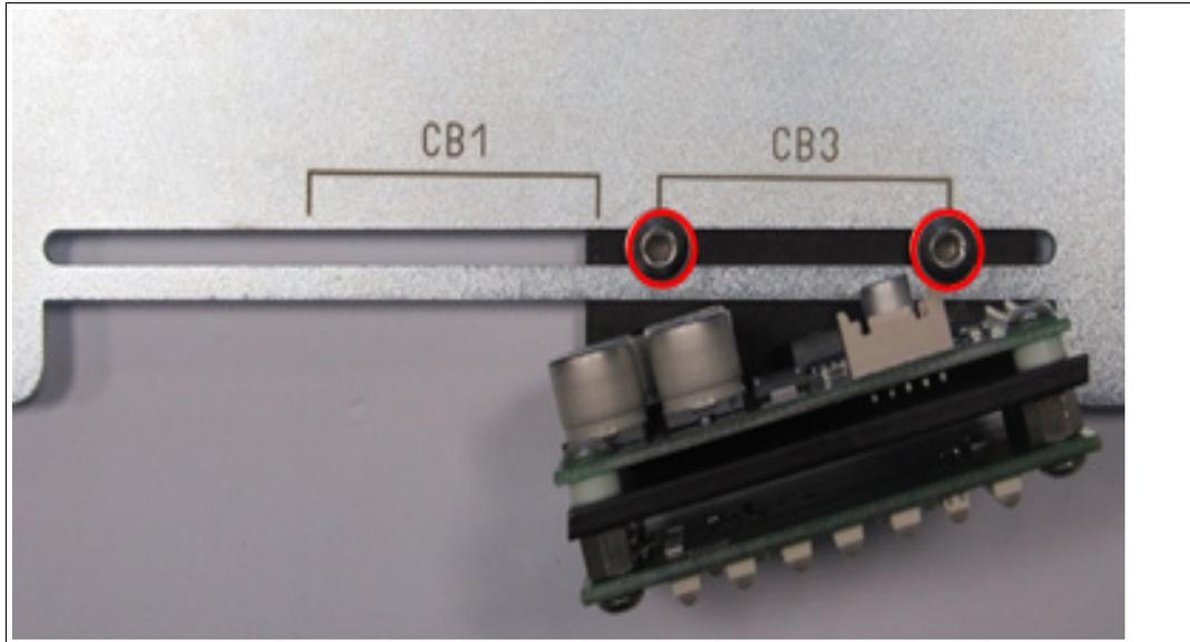
Figure 3.11 Positioning on the rail (CB3)
