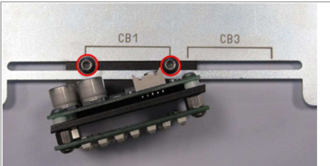
Figure 3.12 Positioning on the rail (CB1)
