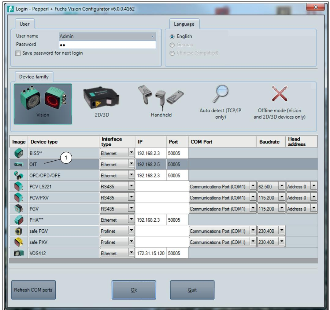
Figure 3.16 Selecting the device
