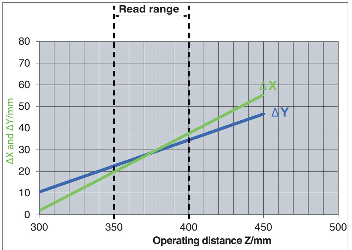
Figure 3.8 Permissible displacement of read-only tag  $\pm \Delta X$  and  $\pm \Delta Y$  depending on reading distance  $Z$
