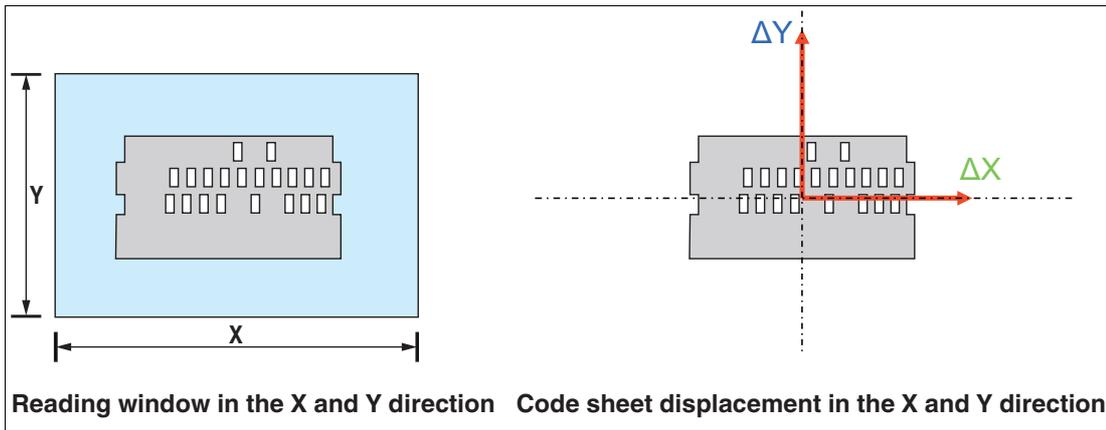
Figure 3.9    X/Y direction for the displacement of OIC-xxxx-CB3 code sheets
