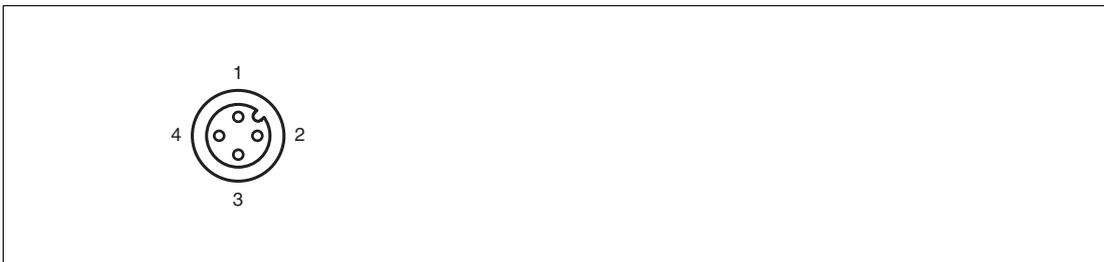
Figure 2.6 Pinout for trigger connection
