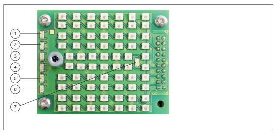
Figure 2.2 Lighting unit of the OIT system
