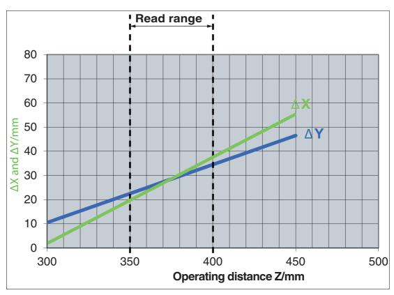
Figure 3.5 Permissible displacement of read-only tag  $\pm \Delta X$  and  $\pm \Delta Y$  depending on reading distance Z
