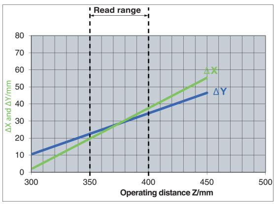
Figure 3.8 Permissible displacement of read-only tag  $\pm \Delta X$  and  $\pm \Delta Y$  depending on reading distance Z
