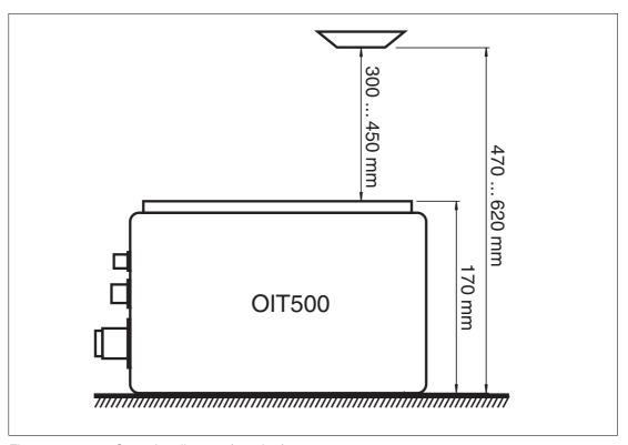
Figure 3.3 Operating distance (top view)
