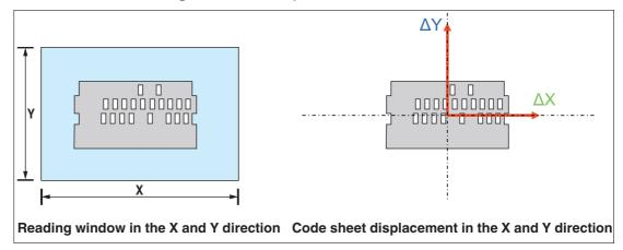
Figure 3.9 X/Y direction for the displacement of **OIC-xxxx-CB3** code sheets
