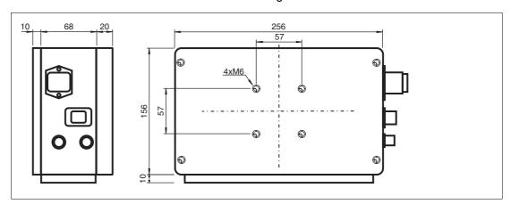
Figure 3.13 Dimensions of the OIT500 system
