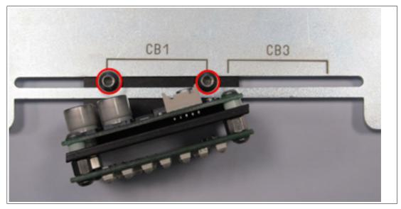
Figure 3.12 Positioning on the rail (CB1)
