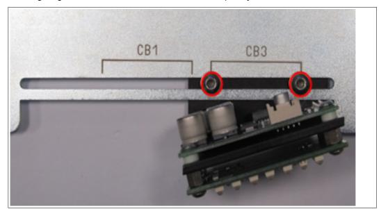
Figure 3.11 Positioning on the rail (CB3)
