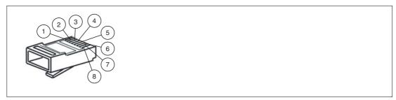
Figure 2.5 Pinout for Network Connection
