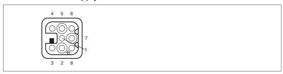
Figure 2.4 Pinout for power supply
