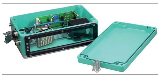
Figure 3.10 Removing the enclosure cover
