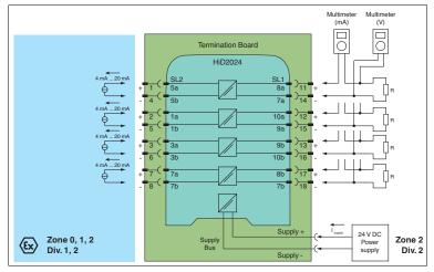
Figure 5.2 Proof test set-up for HiD2024 with analog input function with current source or voltage source output
