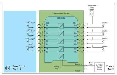
Figure 5.3 Proof test set-up for HiD2024 with analog input function with current sink
