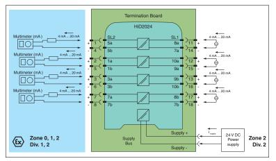
Figure 5.1 Proof test set-up for HiD2024 with analog output function
