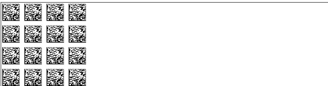
Figure 8.10 The code card assigns the orientation 180° to the read head.
