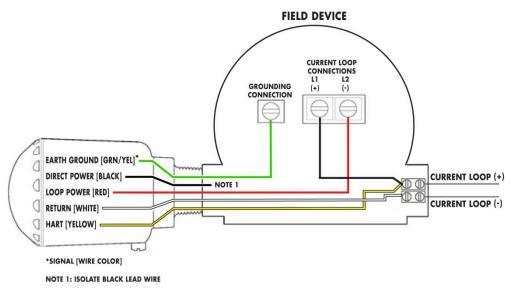
FIGURE 26: Configuration #2 BULLET inserted into the current loop between the FIELD DEVICE negative current loop terminal (L2) and the power source negative terminal.
