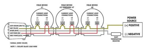
FIGURE 27: LOOP POWER Multi-Drop Configuration
