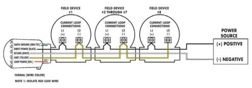
FIGURE 28: DIRECT POWER Multi-Drop Configuration – FIELD DEVICE CONTROL – ON position
