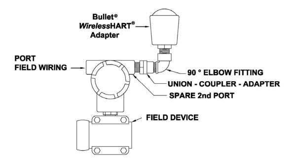
FIGURE 24: Typical BULLET - Field Device installation
